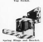
ing drawings. The spring hinge is at the bottom; the pivot and socket at the top. It is very easy to apply this hardware, the only tools necessary being a screw driver and bit brace, or if the top pivot is applied to the top of the gate without mortising, a screw driver only is needed.
