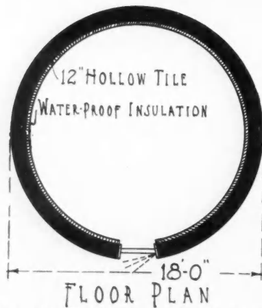
The Circular Tile Ice House Is Built of Silo Blocks Curved to the Proper Circle and Reinforced with Steel Bands in Each Course of Blocks.
