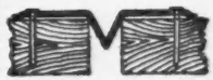
Shows end view of Batten with the joint open and siding contracted. Chief Battens automatically accommodate expansion and contraction.
