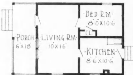
Floor Plan Comfort Cottage. Size 18 by 22 feet.
