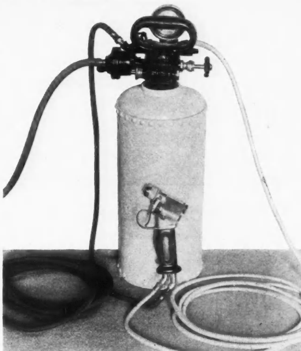
Complete Paint Gun Outfit Which, When Connected to a Suitable Compressed Air Supply by Heavy Tube Leading Off at Left, Will Spray Any Grade of Paint.
