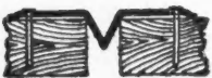
Shows end view of Batten with the joint open and siding contracted. Chief Battens automatically accommodate expansion and contraction.
