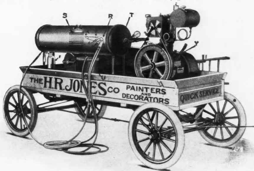
This Outfit is Mounted on an Auto Trailer for Quick Service Onto the Job and Home Again.
