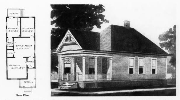
Narrow four-room house, 18 feet in width by 39 feet in length is shown in this design. For a narrow lot it offers the advantage of four rooms with only 18-foot width of building.
