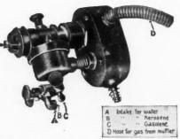
(Continued to page 62.) Carburetor Arranged to Burn Either Kerosene or Gasoline.
