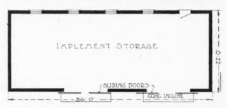
Photograph and Floor Plan of Snug and Substantial Farm Machinery Shed of Hollow Tile. Size is 56 by 22 Feet. Two Pairs of Sliding Doors Make It Convenient to Get Any Implement Out with Very Little Shifting of Other Tools.
