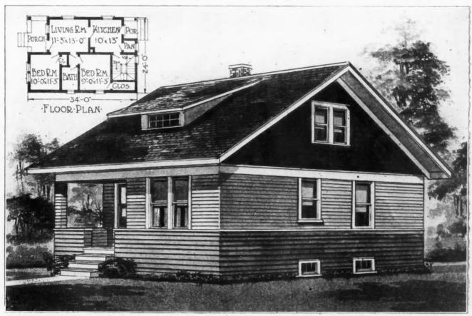
BUNGALOW TYPE COTTAGE. This design, 24 by 34 feet, gives four rooms and bath nicely arranged. Two closets and a pantry are previded. Wide boards for the foundation with narrow siding above and gables shingled, make the exterior attractive.
