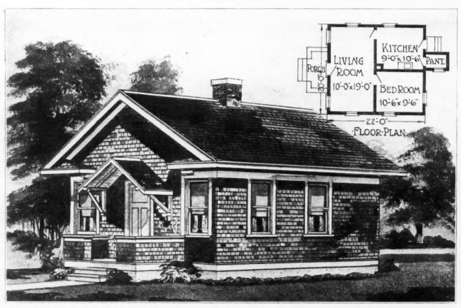
THREE-ROOM SHINGLED COTTAGE. Here is a little gem. Size is only 20 by 22 feet, but no space is wasted. A pleasing exterior is secured at small extra expense.
