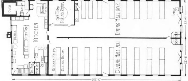
The Floor Plan Shows the Restaurant Building to Be 102 by 45 Feet, Divided Lengthwise Into Two General Dining Halls. At the Rear Is a Good-Sized Kitchen, Laid Out for Efficiency.
