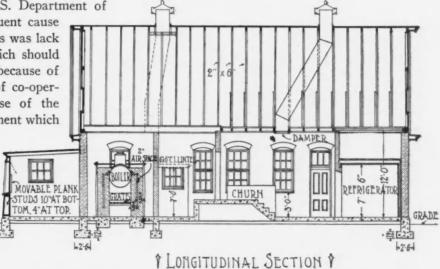
Section Thru U. S. Creamery, Showing Contour of Concrete Floor, Roof Framing, Ventilating Flues, Etc.
