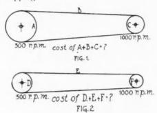
A Narrow Belt Over Large Pulleys May Be Cheaper Than a Wide Belt Over Small Pulleys
