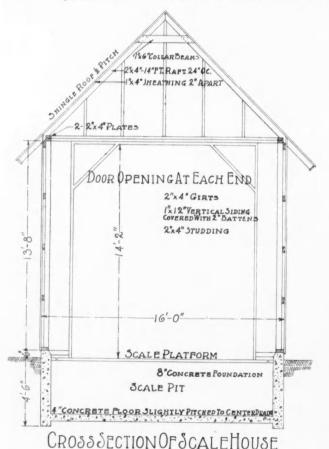
The Concrete Scale Pit Serves as Foundation for the Scale House. The Door Openings Should be High and Broad Enough to Pass the Biggest Load of Hay.
