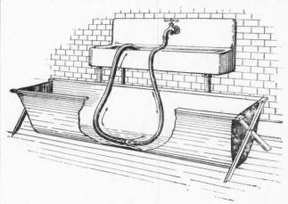
Bath Tub Being Emptied Thru Automatic Device Operated by Water Pressure.
