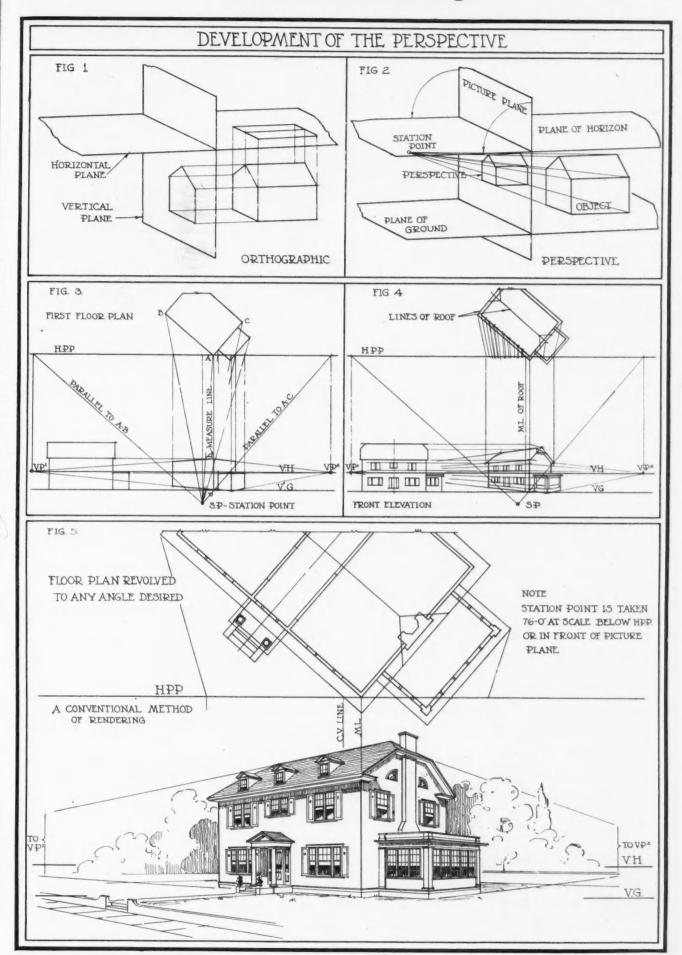
The Fundamentals of Architectural Perspective Drawing; Plate Prepared by Franklin G. Elwood.
