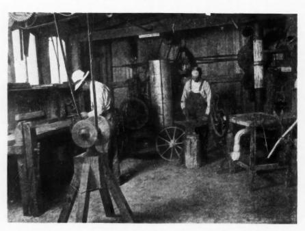
The Farm Shop is Equipped with Forge, Anvil. Power Grindstone, Practical Workbench, and a Good Selection of Blacksmithing and Woodworking Tools.
