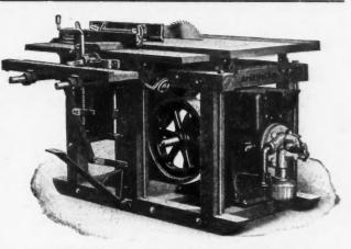
"American" Variety Woodworker with Gasoline Engine Built in. Also supplied with Self-Contained Electric Motor, or arranged for Belt Drive.
