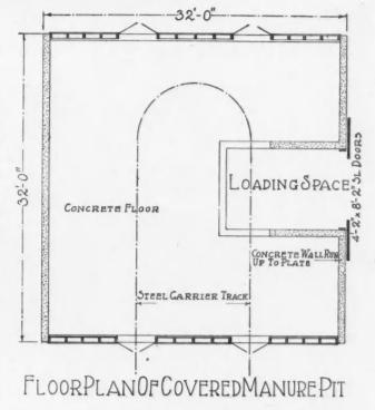
The Overhead Carrier Track Is Built on a Slope so That the Tubs Make the Circuit in and Out Again, Automatically Dumping Inside Wherever Wanted. Gravity Does the Work.
