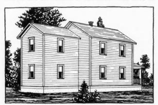
Wrong Method and a Better Way of Roofing an Extension Built Onto the Rear.
