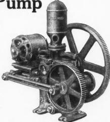
Goulds Fig. 1531 "Form Q" outfit consists of 6 G. P. M. pump with 110 or 220 A. C. or D. C. motor—or with 32 volt motor for operation on farm lighting systems. For pressures up to 43 lbs.
