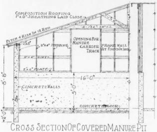
The Manure Shed Has an 8-Inch Concrete Wall 5 Feet High Across the Ends, and 8 Feet 8 Inches on the Sides.
