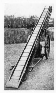
Close Up View of Portable Scoop Conveyor.
