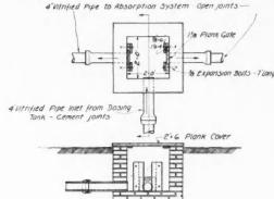
Fig. 7. The Diversion Chamber.
