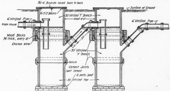
Fig. 4. A Septic Tank of Vitrified Pipe Is Simple to Construct and Gives Everlasting Service.
