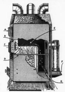
The Hess Pipe Furnace With separate pipes and registers
