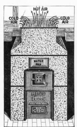
The Hess Pipeless Steel Furnace One register only -serves for both hot and cold air
