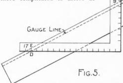
from the outer surface of the rafter. The steeper the roof the greater or more pronounced the backing will be; and consequently the error if not understood by the framer, in making the proper allowance.
