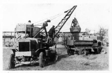
The "Winther" Truck and Mounted Hoist Delivering the Clam-Shell's Load to Another Truck.
