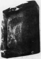
B and C-Two Varieties Without Copper. Loss, 42 3/10 Per Cent. Loss, 47% Per Cent. WHAT THE TEST OF STEEL BOOFING WITH AND WITHOUT COPPER SHOWED.
