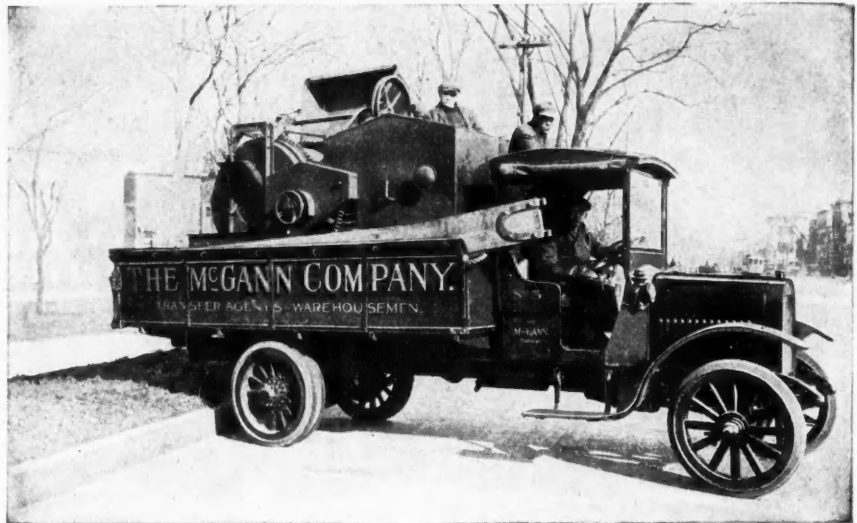
Newark, N. J., Contractors Employ the McGann Company to Quickly Transport Their Equipment to and from the Job. Here Is a Concrete Mixer Loaded in a 3 1/2-Ton "Acme" Truck.
