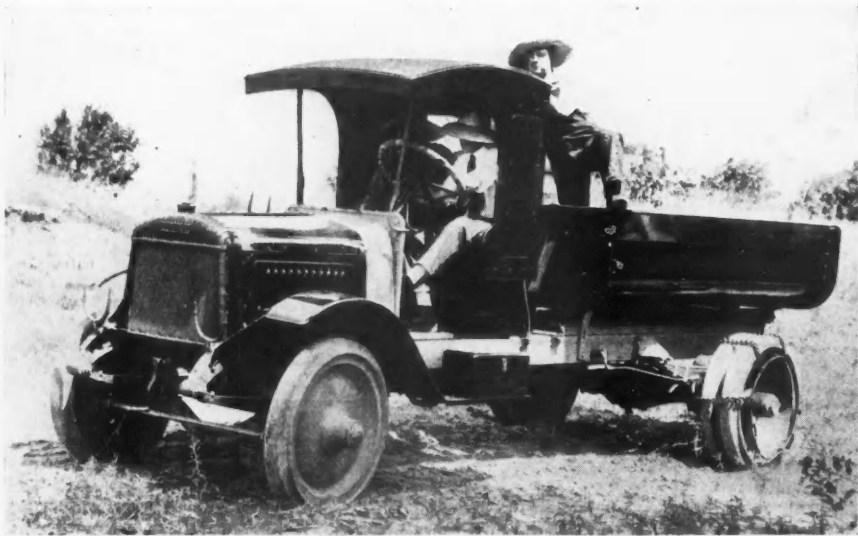
Here is a 3½-Ton "Republic" Truck, Equipped With a Dump Body, Designed to Do the Work Required by Building Contractors.
