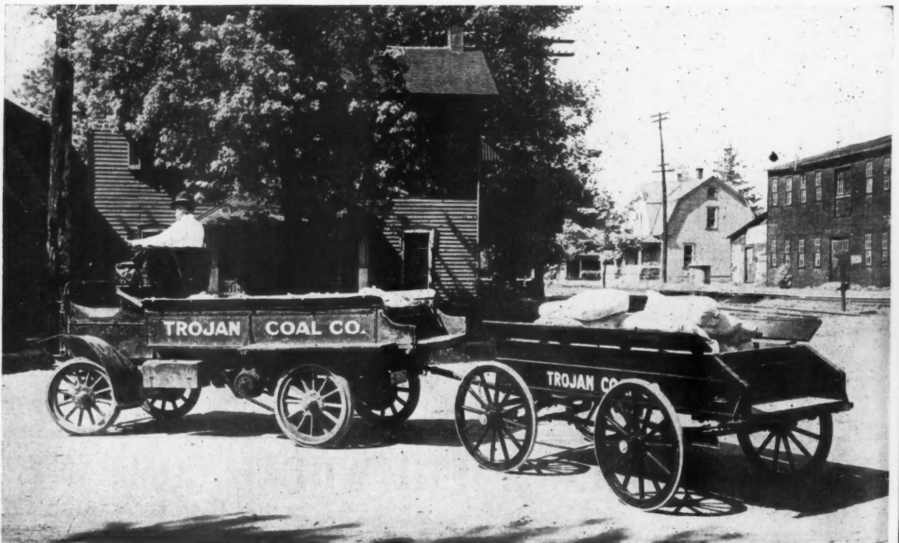
This Small Four-Wheel "Miami" Trailer Doubles the Capacity of the Light Truck in Hauling Cement and Other Like Building Materials.
