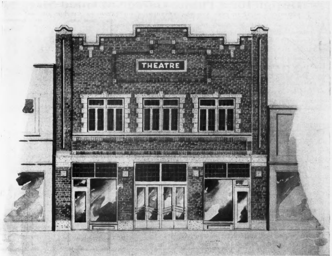
Front Elevation of a Theater Seating About 700 People. It is of Standard Brick Construction and Fireproof. Stores on Either Side of the Entrance Add to the Owner's Income. This Is an Excellent Small Theater Design.
