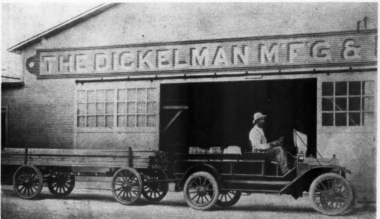
The Dickelman Manufacturing & Lumber Co., Forest, Ohio, Are Enthusiastic Over the Trailer as a Means of Cutting Lumber Delivery Costs. The Illustration Shows One of Their "Trailmobiles" Attached to a Small Truck and Carrying a Good-Sized Load of Lumber.
