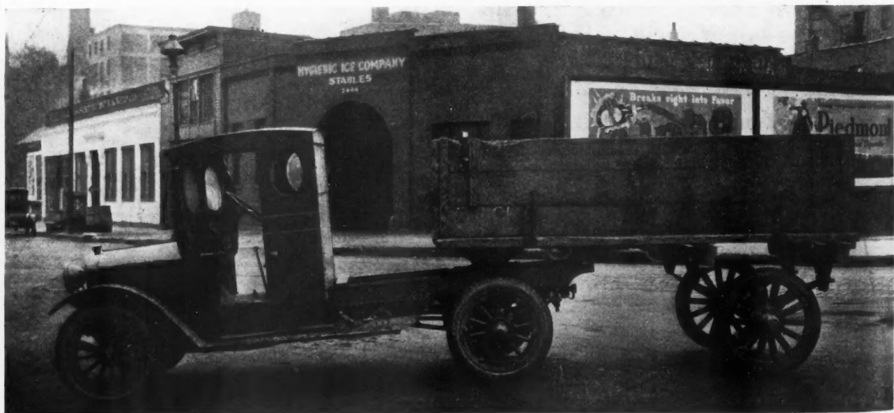
The "Reo" Tractor and "Martin Rocking Fifth Wheel" Trailer That Gave Such a Good Account of Themselves in Hauling Brick for the Hydraulic Press Brick Co., Chicago.
