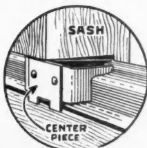
Center Piece to Protect Opening Between Casement Windows.
