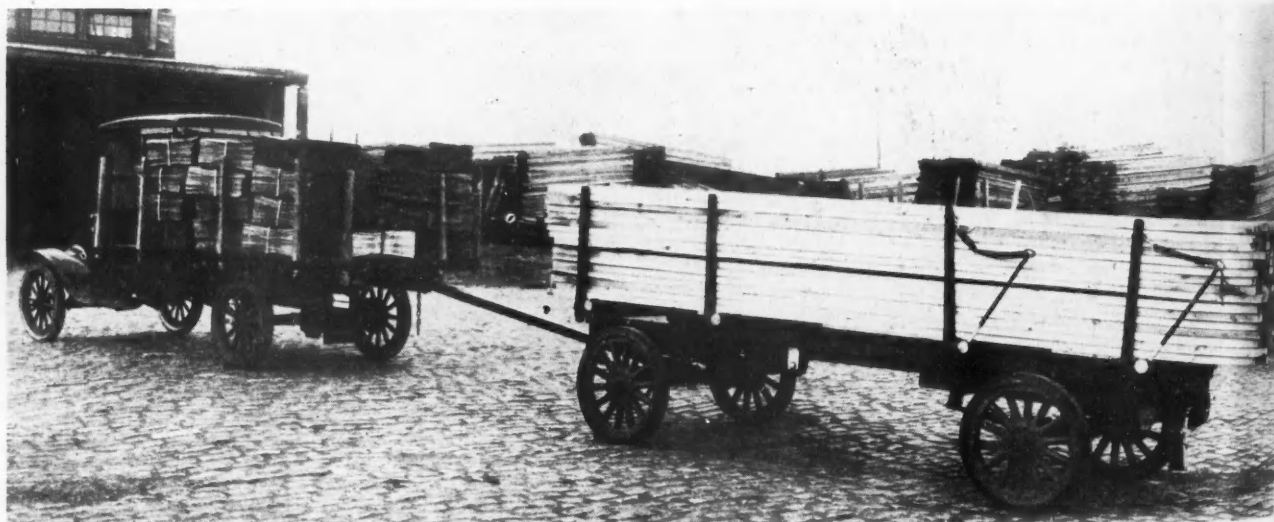
Four-Wheel Trailers More Than Double the Capacity of Light Motor Truck of Charles H. Finch & Co., Brooklyn, N. Y., with a "Trailmobile" Attached, the Truck Loaded with Shingles and the Trailer Carrying a Good-Sized Load of Lumber.
