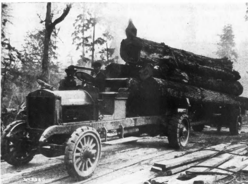
"Diamond T" Motor Trucks Now Penetrate the Dense Forests on the Pacific Coast, Where They Are Used to Haul Logs to the Mills. The Trucks in the Illustration Are Owned by the James D. Esary Co., of Itsalady, Wash. When the Ground Is Too Soft to Hold Up Heavily Loaded Trucks, Tracks Are Formed on Boards Over Which the Trucks Run Smoothly and Speedily. Trucks Have Proven to be a Rapid and Economical Means of Log Hauling.
