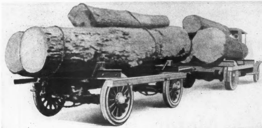
Here is the 3\frac{1}{2} -Ton "Acme" Truck and the "Trailmobile" of Equal Capacity Used by the Amos Lumber Co., Edinburg, Ind. The Truck and Trailer Are Loaded with 19,000 Pounds of Logs and Haul Them Over the Country Roads Near Edinburg.
