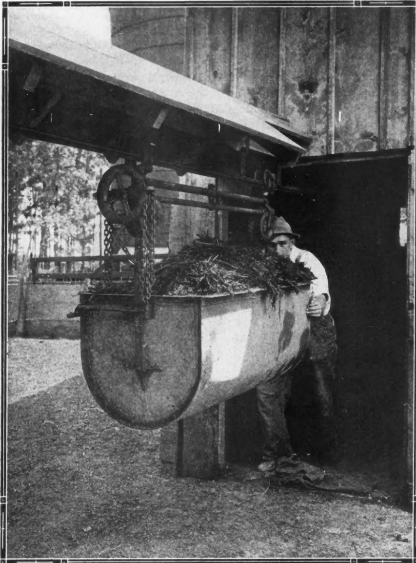
The Litter Carrier Is a Great Saver of Labor in the Modern Dairy Barn. This Is One Piece of Equipment That the Present-Day Farmer Needs Most of All.
