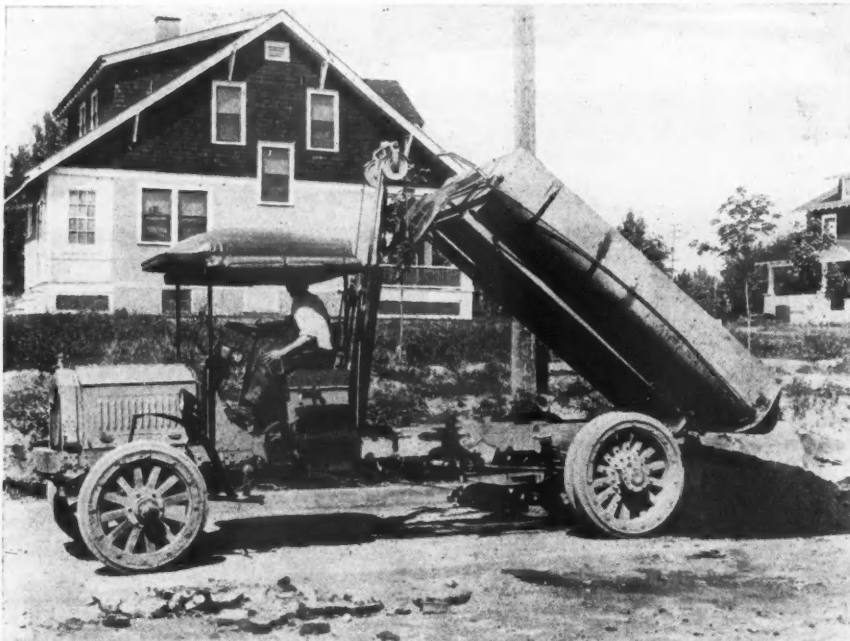
Three-Ton "Packard" Truck, Equipped with a Dump Body, Designed Especially for Hauling Building Materials. This Truck Is Owned by the Schenectady Construction Co., Schenectady, N. Y., and is Shown Delivering a Load of Sand to the Building Job. This Body Enables the Truck to Be Unloaded with Great Speed, Saving Time and Money in Hauling.
