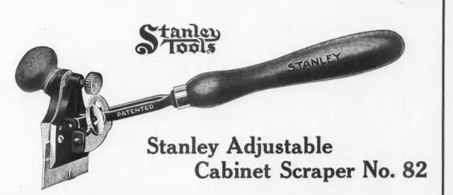
Its form is such as to give a natural and easy position to the hands and it balances well in working. The handle is adjustable and can be tilted to give the blade any angle desired.
