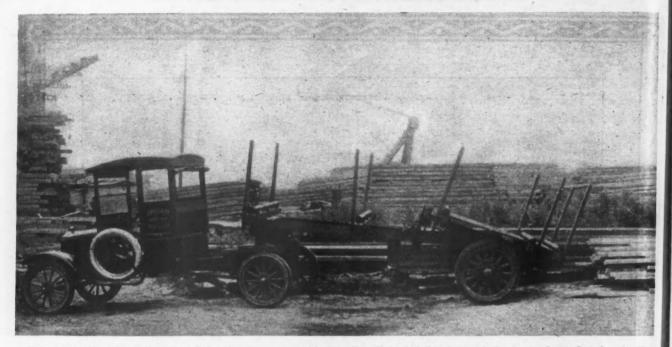
Three-Ton "Semi-Trailmobile" with Lumber Dump Just After It Has Unloaded Lumber and Ready to Start Out for Another. This Trailer Is Owned by Church E. Gates & Co., New York City, Who Have Seven More in Active Use, Four Semi-Trailers and Four of the Four-Wheeled Type.
