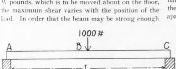
Fig. 8. Simple Beam with Central Load.
