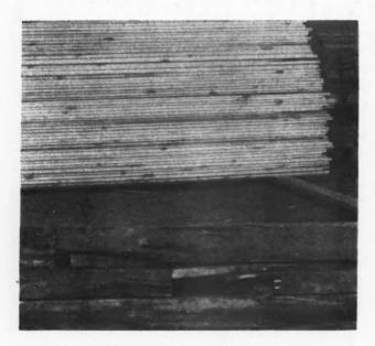
Note the Contrast Between New Lumber and Wood That Has Been Attacked by Fungl. Wood Preservers Have Been Used with Effect to Stop This Wood Rot. The Fungl Attack the Wood Near the Ground. Creosote Oil Has Properties Which Kill Germs and Lengthen the Life of the Wood.
