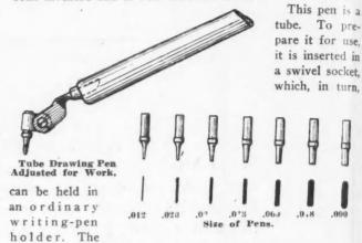
tube pen is then filled with a pipette or quill. While being used it should be held perpendicular to the paper, the swivel socket being adjustable to suit the usual position on the hand. These tube-pens are made in seven sizes, from 0.012 to 0.090 inches, and are used for either free-hand or ruled work.
