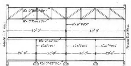
Suggested Truss for Building with Hollow Tile Walls. It Is Made Up of Built-Up
