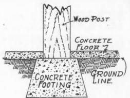
Diagram Showing Position of Posts on Concrete Footing. Timber Experts Advise Setting Posts on Top of Floor and Treating Bottom with Tar Creosote.
