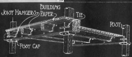
SEMI-MILL CONSTRUCTION, BEAMS IN HANGERS.
