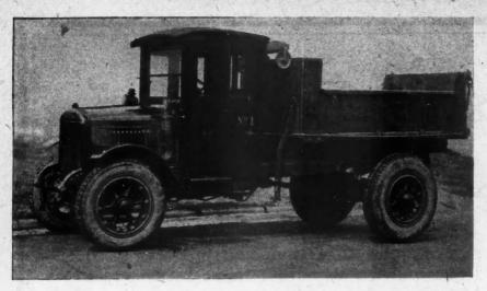
Pneumatic Tires and a Special Loading Body for Hauling Building Materials Are Two Features of This New "Republic" Truck Owned by M. J. Watkins, Contractor in Grand Rapids, Mich. He Finds it Cuts Costs by Its Speed and Labor-Saving Dumping Device.
