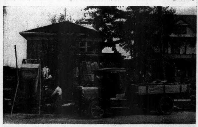
Three and One-Half Ton "Gramm-Bernstein" Truck with Special Square Cornered Dump Body to Speed Up Loading of Brick, Owned by the Lima Construction Co., Lima, Ohio. The Side Boards Are Removable to Form Platform Body When Hauling the Concrete Mixer or Other Heavy Machinery.
