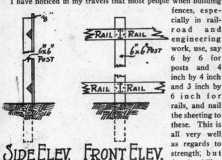
change which would save one-half the amount of lumber. For instance, take rails 4 by 4. If they are ripped diagonally this will give you a three corner or triangular rail and would be used as shown in Fig. 1. The method of fixing the posts as shown in Fig. 2, gives one a substantial fence and also a rail that will shed water and prevent rot. The rail will be 27/8 by 53/4 inches wide. This applies equally well to picket fences.
