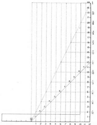
Fig. 1. Figures Representing Rise Given Common Rafter to a One-Foot Run.
