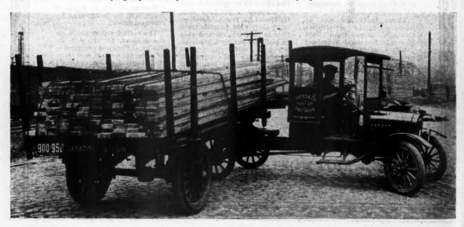
This Picture Shows the Adaptability of the Trailer for Making Short Turns in the Lumber Yard. This "Trailmobile" Is On of Several Owned by Church E. Gates & Co., New York City. The Jack-Knife Frame Enables the Driver to Dump the Lumber is a Few Minutes.
