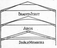
Types of Simple A-Shaped Trusses.
