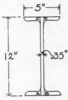
Fig. 9. Beam Showing Shearing Area.
