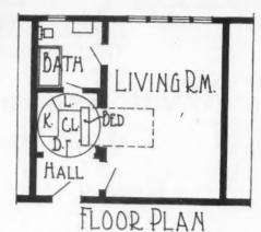
Figor Plan of New Space-Saving Apartment in Which Revolving Compartment Is Installed.
