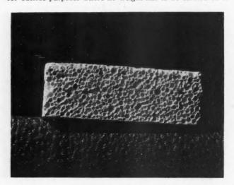
Cross Section of Concrete Slab Showing Porous Character of Material. These Air Holes Help to Make it an Insulating Material to Be Used in Partitions. It is Manufactured in Thin Slabs 24 by 32 Inches and One Inch Thick.
