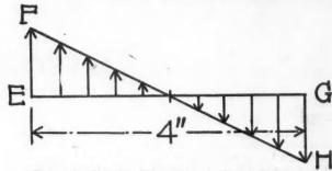
Figure 3. Showing Fibre Stresses Due to Bending.
