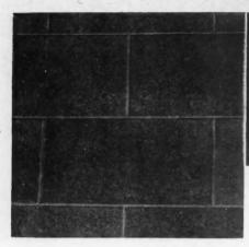
Figure 7. Block Surface Produced with Facing of Cement, White Marble, Gray and Black Granite and Mica, Washed with Fog Nozzle on Removal from Mold.
