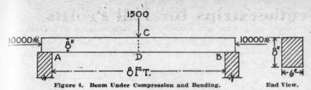
latter stress. But with cast iron for which a safe working tensile stress is only 3,000 pounds per square inch, while the safe working compressive stress is 15,000 pounds per square inch, both fibre stresses must be carefully consid-
