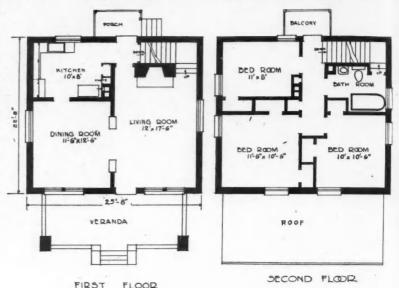
First and Second Floor Plans of Efficiently Designed Brick Home. It Contains Six Large Rooms,
