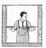
the rule to within 6 inches, or less, of the distance between the points. Extend the brass slide by push button. Add the measurement on the brass slide to that shown at extreme end of rule, which gives the exact distance. The extension slide is also admirably adapted to determining depth of mortises, etc. The boxwood sections are somewhat heavier than those
