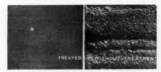
Concrete as It Appeared Before and After Treatment by Special Hardener. This Is a Chemical Preparation That Is Applied After the Surface of the Concrete Is Set.
