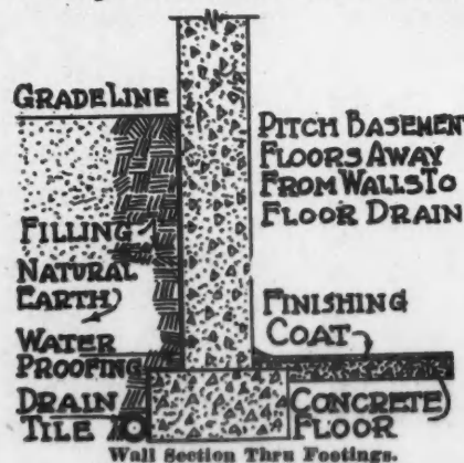
Wall Section Thru Footings.
