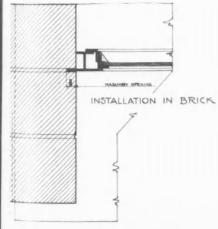
Febrisco Solid Steel Basement Sash is made in 3 standard sizes, in both 2 and 3 lights and meets all practical requirements. It can be installed in brick, masonry, cement block, tile or concrete walls.
