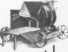
Wolverine half-bag capacity low charger—equipped with 3 HP horizontal gasoline en-gine with magneto— engine housing—sells for \$325.00, f. o. b. factory. May be equipped with batch hopper.
