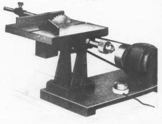
Small Bench Machine for Light Work in Wood and Metals
