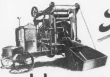
Sizes 21 and 14 cu. ft. mixed material—four cylinder truck and tractor type gasoline
