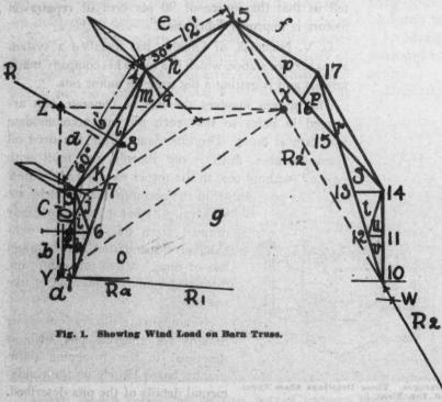
z draw a line equal and parallel to AF. This is the resultant R of all the wind loads.
