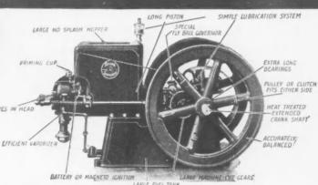
All Adjustable Parts are Easily Accessible and Once Adjusted can be Locked in Position
