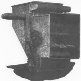
Mechanical Stucco Machine for Applying Stucco to Walls. The Material Is Poured in Thru the Top and Sprayed Out by Turning the Handle on the Side.
