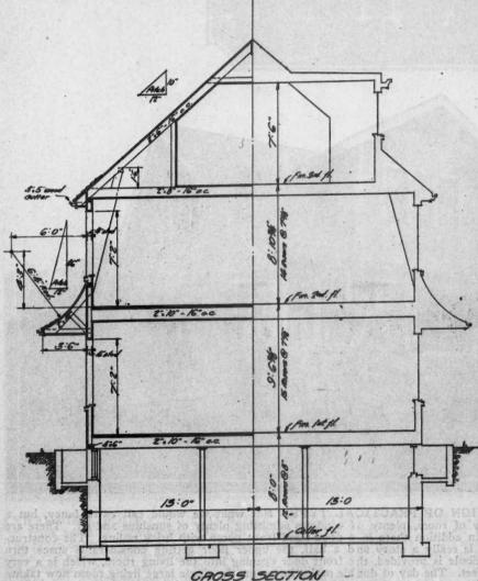
Cross-Section of Gambrel Roof House Showing Details of Construction.
