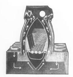
This cut shows how the FarQuar Furnace is scientifically designed to gently warm the cool, fresh air instead of rendering it lifeless and devitalized through super-heating.
