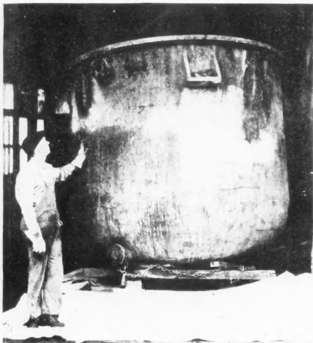
Huge Tar Kettle Which Was Repaired by Oxyacetylene-Welding Process at a Saving of $1,200. The Kettle Weighs 1,300 lbs. and Had Two Ruptures in It, 18 and 26 Inches Long.
