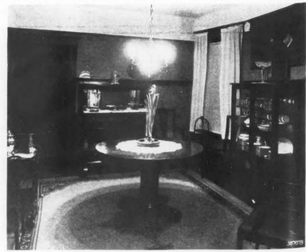
The Luminaire Shown Here Makes the Table Bright and at the Same Time Provides General Room Illumination. A 75-Watt Lamp Is Used in the Center Light and 25-Watt Bulbs in the Others.
