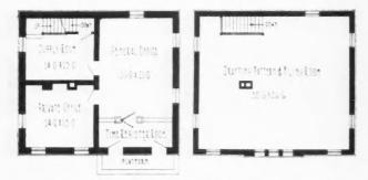
First Floor Plan at the Left. The Second Floor Is One Large Room Used for Drafting and Filing Purposes.
