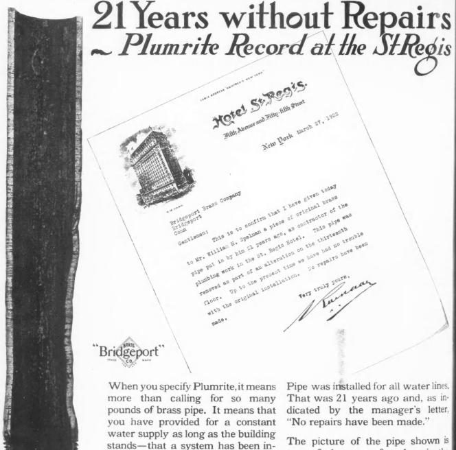
Piece of pipe referred to in the accompanying letter. Note full threads and full thickness of the wall throughout the length. Also the softness of length. Also the softness of the pipe as evidenced by the crushing of the sides with the pipe tongs when removing it. The roughness on the inner surface is a slight scale forma-tion and not corrosion.
