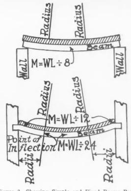
Figure 2. Showing Simple and Fixed Beams Bent Under Load.
