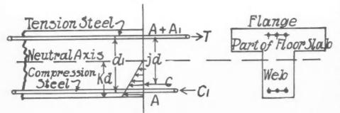
Figure 4. Showing Resisting Moments in Beam with Compressive Steel.
