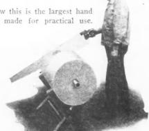
Said to be Largest Hand Saw Ever Made for Practical Use, Is 48 Inches Long. Used to saw rolls of paper.
