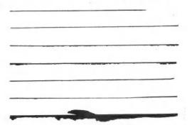
Fig. 6. Various Types of Faulty Lines to Be Avoided.
