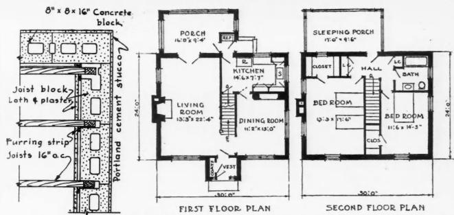
Cross Section of Concrete Block Stuccoed Wall, Showing Use of Joist Blocks and of Furring Strips, Giving an Air Space Between the Inner Block Face and the Lath and Plaster. This is good practice in concrete block work, the same as in brick or natural stone. The floor plans of this house show four large rooms downstairs, and two bedrooms, bath and sleeping porch upstairs.
