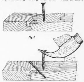
Fig. 2. How to Raise Broken Floor Board.
