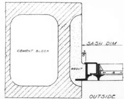
Fig. 2. Detail of Window Head Construction, Concrete Fig. 4. Detail of Window Jamb, Concrete Blocks and Steel Sash.
