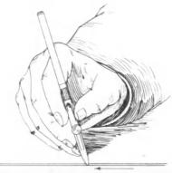
Fig. 7. Correct Method of Holding Ruling Pen.
