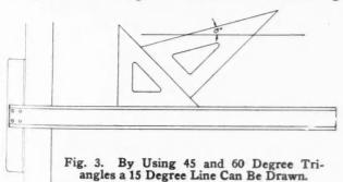
ure 2, the arrows guiding the direction of the stroke. Now by using the two triangles in combination, we can get angles of 15, 75 and 105 degrees. For instance, if the draftsman wishes to draw a line making 15 degrees with the horizontal (or line of the T-square) he first sets the 45 triangle against the T-square and then the 60 degree against the 45 in the manner shown in Fig. 3. This leaves the difference between 60 and 45, or 15 degrees, the angle sought.
