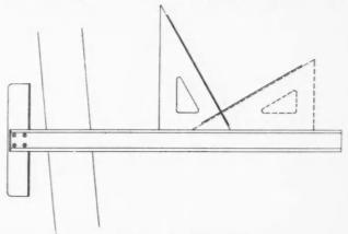
Fig. 5. Using a 60 Degree Triangle to Draw One Line Perpendicular to Another.
