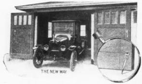
A Convenient Stopper for a Garage Door Drops Down and Grips the Driveway. A simple, inexpensive idea that guards against dented fenders or more serious damage.
