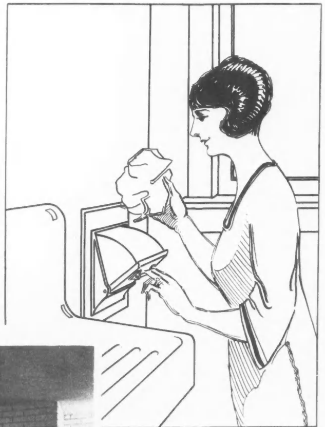
The Kitchen View of the Garbage Incinerator. A neat hopper door (always closed) admits to the flue.
