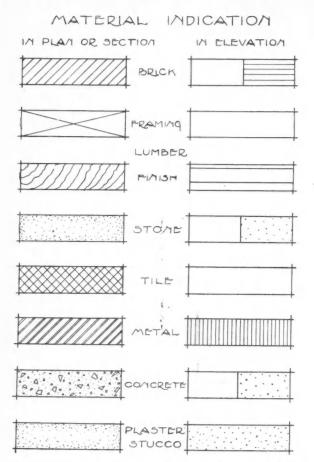
The System of Material Indication Should Always Be Clearly Sufficient to Define the Materials Which the Builder and Contractor Is Expected to Furnish.
