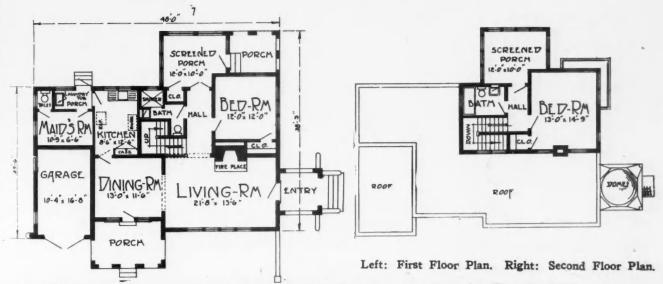
The Inbuilt Garage Is a Feature in This Plan, as It Is with the Others. Notice the provision made for porches. Seems to us, if we were in Florida, our house would be a porch with a room attached.
