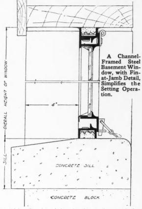
inches thick. Set the window in place and press it firmly into the cement until it is plumb and rests firmly on the two wood blocks.
