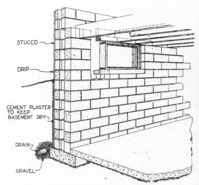
Detail of Concrete Block Construction.
