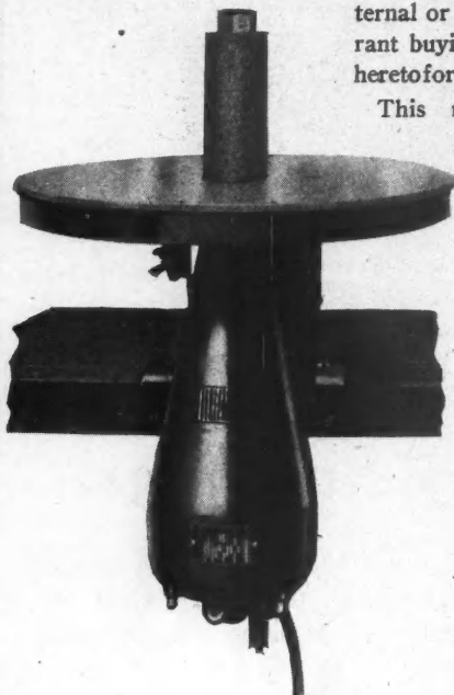
A Good Spindle Sander for the Woodworking or Pattern Shop. Motor-driven and very inexpensive.
