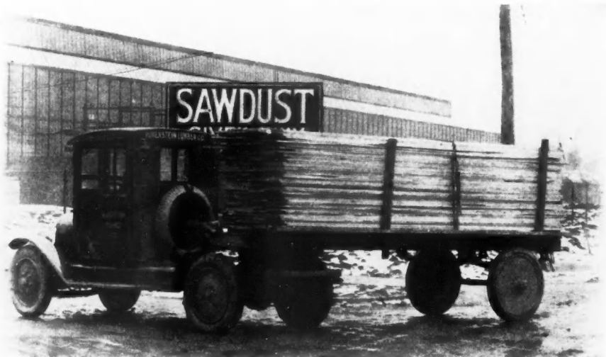
This Method of Handling Lumber Deliveries with Trailers and a Fast, Short-Coupled Truck for Hauling Them Has Been Found Very Satisfactory by a Chicago Lumber Dealer.
