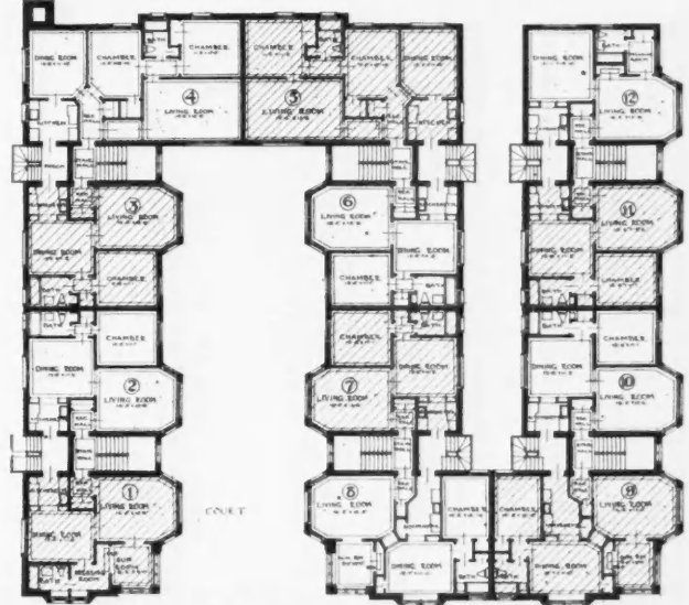
A Typical Floor Plan of The Tudor Manor Shows a Typical Arrangement of the 36 Three to Five-Room Apartments.
