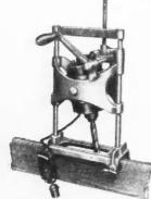
This Little Machine Makes Possible Quick, Accurate Mortising for Door Locks, by Unskilled Workmen.
