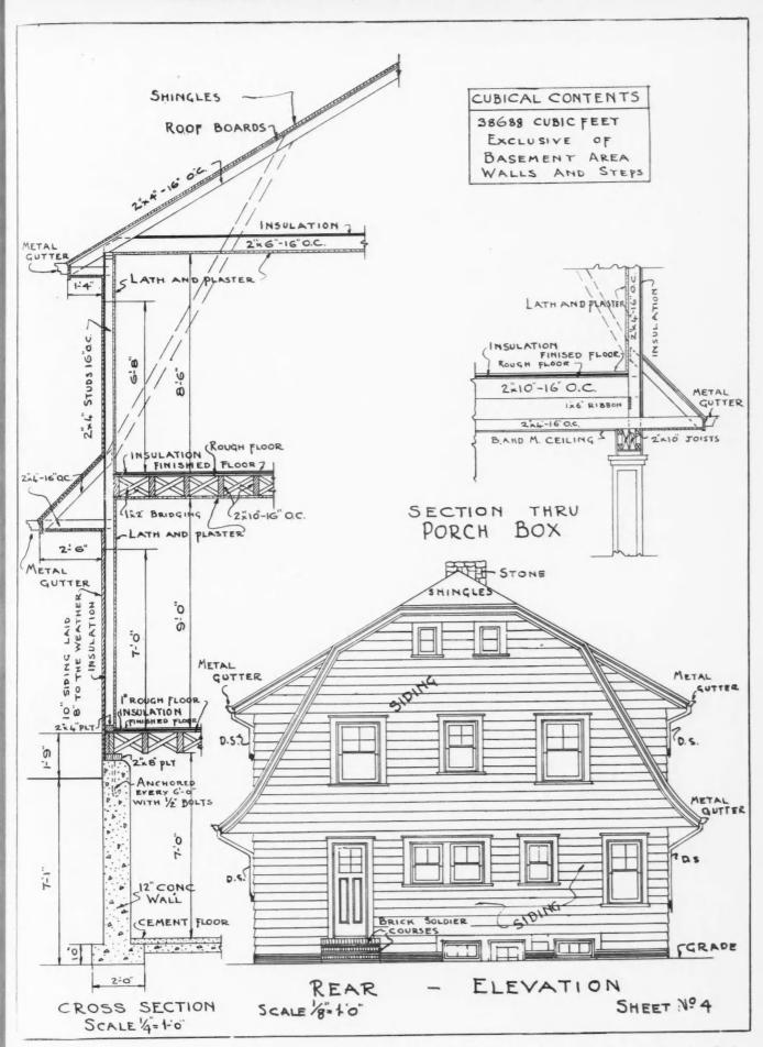
The Good Construction of Our Front Cover Home Is Illustrated in This Cross-Section Detail, One-Quarter Inch to the Foot.
