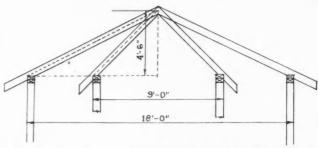
Fig. 4. How Roofs of the Same Height May Have Different Pitches, Depending Upon the Width of the Roof.
