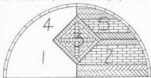
This Brick Panel Was Laid on the Ground in Five Sections Which Were All Ready to Put in Place Without Delay When the Wall Reached the Proper Point.
