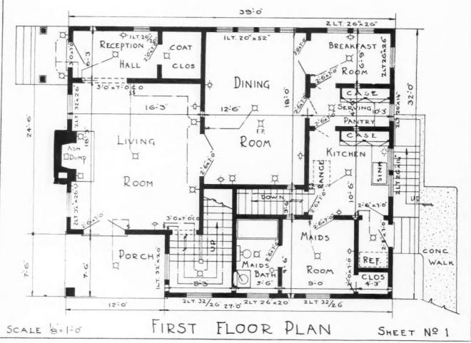
Working Drawings to One-Eighth Inch Scale of First Floor Plan and Front Elevation of the Dutch Colonial Home Illustrated in Full Colors on Our Front Cover.
