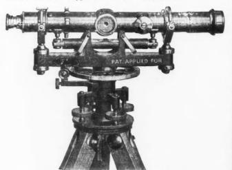
A Convertible Level, Particularly Adapted to the Needs of the Contractor and Builder, Is Equally Serviceable for Laying Out Surface Work and for Vertical Sighting.
