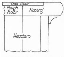
This Method Makes a Solid Job with Joints That Will Not Open from Shrinkage.
