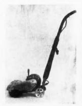
A Small Sanding Machine Which Can Be Quietly Changed Into a Polishing Machine Serves a Double Purpose.
