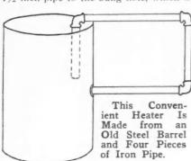
This pipe extended out about 4 feet, then turned up to just above the level of the top of the barrel, again turned toward the barrel and finally down into it. A fire built under this pipe heats the water in the barrel in the same way as a
