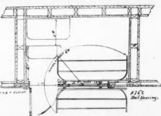
This Diagram Shows How the New Bed Can Be Swung in a 24-Inch Radius Even When Equipped with Box Springs.
