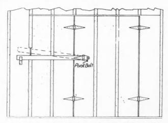
Connecting the Bar by Means of a Pivoted Strap Hinge Permits It To Be Swung Out When the Door Is To Be Opened and So Easily Clear the Batten.
