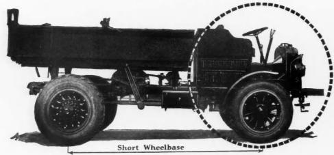
The contractor's special 3-ton Autocar dump Truck
