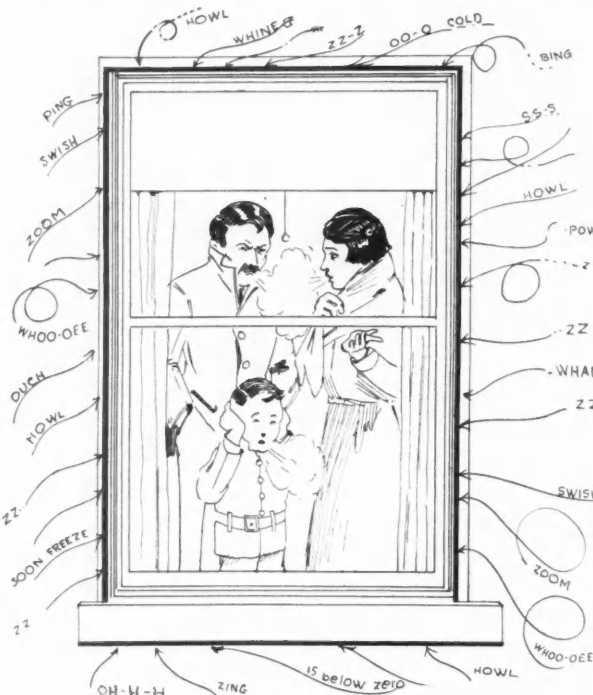
Winter Winds That Enter Through Uncalked Window Frames Amount in Coal to 75 Pounds Per Foot of Crack \frac{1}{4} Inch Wide Where Average Winds Are 15 Miles Per Hour.
