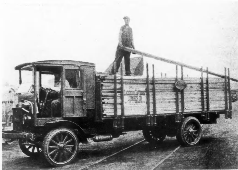
4-cylinder KA model Autocar. The extra long wheelbase and engine-under-the-seat design give maximum body space for extra long loads yet keep the turning radius at a minimum.
