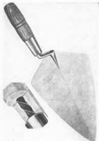
A New Type of Spiral Tang Locks the Handle Securely to the Blade of This Trowel.
