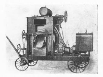
A Worm Speed Reduction, in Place of the Usual Gears and Shafts or Chains and Sprockets, Is the Most Conspicuous Feature of This New Concrete Mixer.
