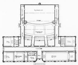
Ground Floor Plan of High School at Cheyenne Wells, Colo. A boiler room is located beneath the fireproof gymnasium stage.
