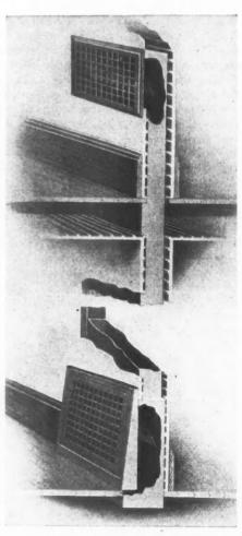
Fig. 1. Sectional View of Warm Air Leader Duct, Baseboard Register and Wafer Type Wall Register.
