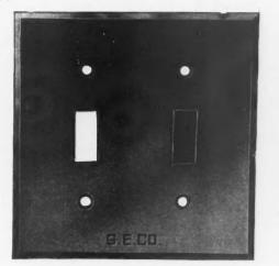
(1/2 actual size) Cat. No. GE1702 Two-gang Plate with GE2331 Removable Bull's Eye, for Switch and Pilot Lamp Receptacle 0.040-in. Metal The combination of switch, pilot lamp and convenience outlet is recommended for the connection and control of heating appliances (for the kitchen principally).
