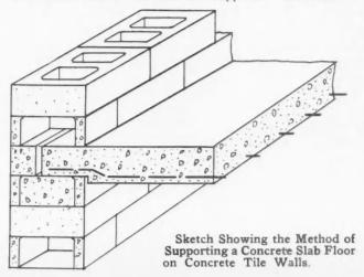
"temperature" reinforcing in all cases consists of ¼-inch round, or deformed bars, space 12 inches center to center, approximately 1¼ inches below the upper surface.
