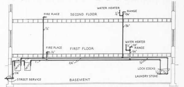
A Two Family Home, Showing Fireplace Connection, Also Range and Tank Water Heater Connection in the Kitchen of Each Flat.
