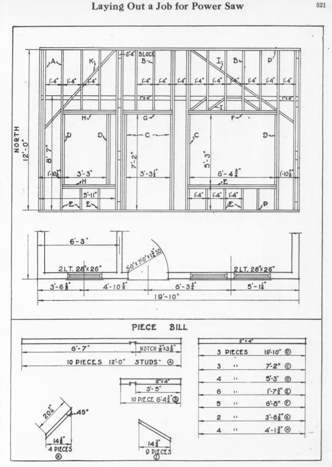
This Sketch Shows How to Use the Floor Plan for Making a Framing Detail and Drawing Off a Piece Bill. With this piece bill, the men at the power saw can most efficiently cut the necessary pieces.
