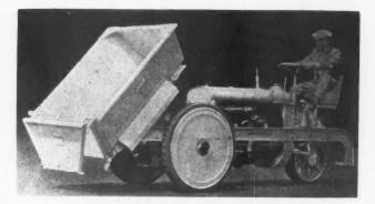
On Soft or Rough Ground This Hopper Dump Bod Mounted on a Fordson Will Be Found a Most Effectiv Piece of Equipment.
