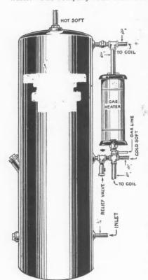
This New Water Softener Is a Non-Regenerating Type and Ordinarily the Eliminating Material Should Last About Four Years.
