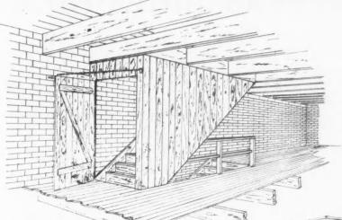
Unprotected Floor Openings Are Another Serious Fire Hazard. Stairways should be protected by an enclosure such as shown.
