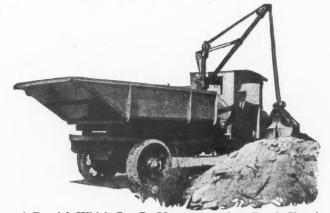
A Derrick Which Can Be Mounted on Any Truck Chassis Is Made in Two Sizes, 1,000 and 1,500 Pounds Capacity, and Is Adapted to Hoisting, Loading and Digging.
