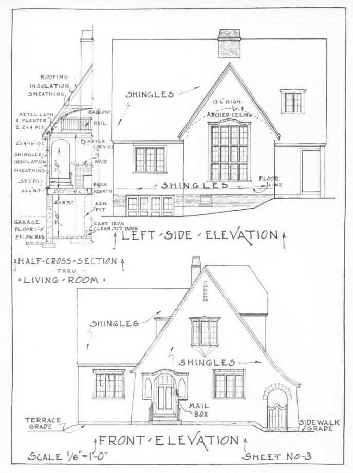
Left and Front Elevations of Our Front Cover Home Show the Relation of Garage to Grade Line, the Arch of the Living Room Ceiling and the Treatment of Entrance and Gateway.
