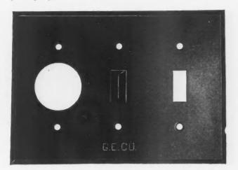
(1/2 actual size) Cat. No. GE2456 Combination Plate with GE2331 Removable Bull's Eye, for Switch, Pilot Lamp Receptacle and Single Convenience Outlet 0.040-in. Metal
