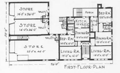
The problem in design offered by a site and building of this character is mainly to utilize the rear half of the lot and make it productive of profitable revenue. This side street being residential, has led to the design of a rear wing which is purely residential in character.
