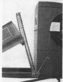
This Simple, Reliable, Hand Hoist Increases the Range of Use of the Ford Steel Truck Body.
