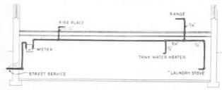
No. 1. A Simple Piping Plan for a One Family Home, Showing (No. 1) Opening in Fireplace, (No. 2) Range, (No. 3) Tank Water Heater, (No. 4) Laundry Stove. tion of a modern cabinet range, good water heater, space heaters and other efficient devices adds greatly to the value —and salability—of the house.
