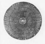
Outer line on this recording thermometer chart shows constant temperature downstairs, day and night, for the entire week ending Feb. 7. Inner line shows outside temperature varying from 16° to 4° to 30° above zero.
