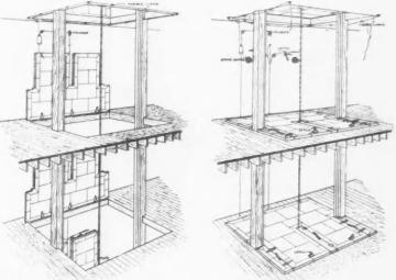
Insurance Companies Demand That Floor Openings Shall Have Protection with Fire Resistance at Least Equal to the Resistance of the Floor Itself.
