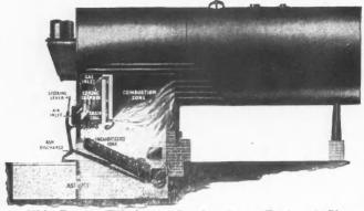
This Burner Eliminates Smoke, Saves Fuel and Gives a Greatly Increased Fuel Efficiency Without Requiring Special Care.
