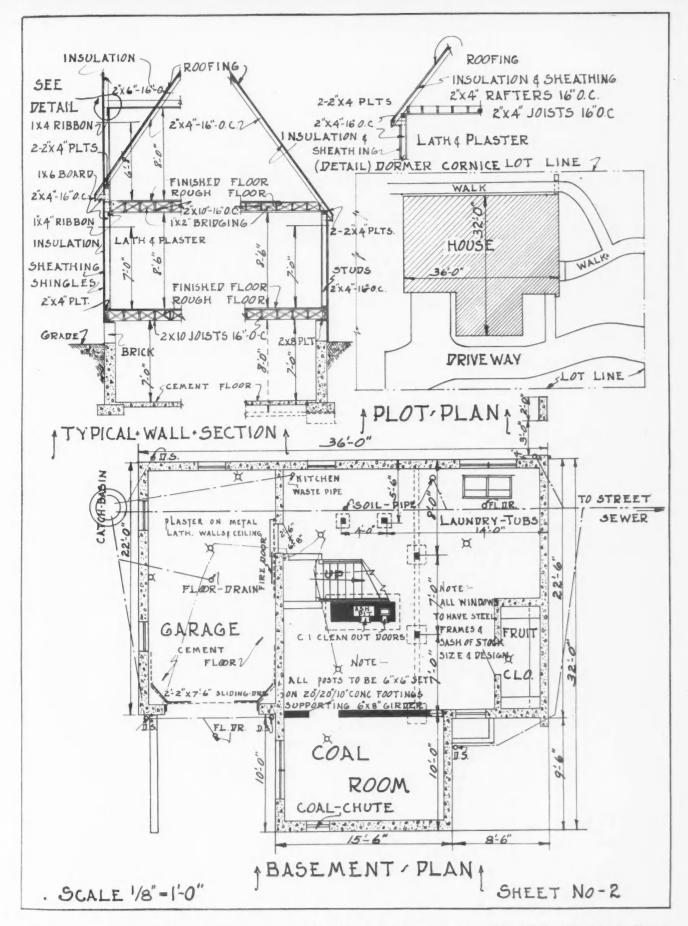
A Garage Is Built into the Basement in a Most Convenient Fashion, Being Accessible Without Going Outside the House. Above are details of wall and roof while on succeeding pages are the elevation drawings.
