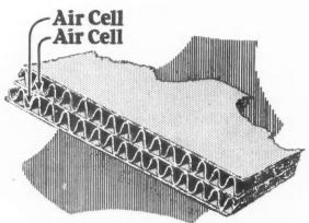
Each ply waterproofed under K-B process patents, by embedding layer of water-proofing compound midway between outer surfaces.
