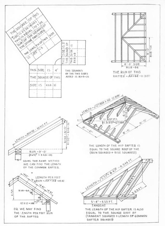
On Page 412 the Method of Calculating Rafter Lengths by Means of Square Root Is Discussed and Above Are Shown a Group of Drawings Which Illustrate the Application of the Method to the Actual Work of Roof Framing as Well as the Basic Rule for Finding the Length of the Hypotenuse of a Right Triangle by Means of Square Root.
