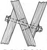
The Units of This Roof Are Bolted Together with Standard Bolts Which Take Up All Shrinkage.
