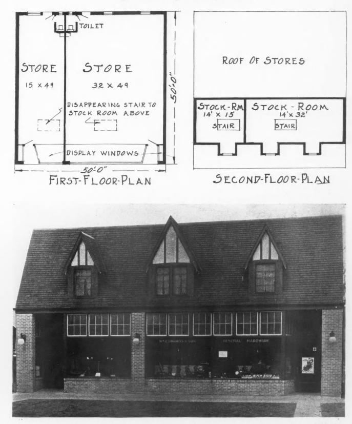
This Lot Being but Fifty Feet in Depth, Small Stock Rooms Are Provided on the Attic Floor Above. Reference to the plan shows that disappearing stairways conserve profitable space in the stores at a minimum cost.
