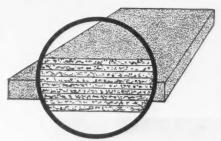
Close examination shows the evenly distributed fine layers of asbestos fibre in the shingle. This fibre is the binder that gives the shingle its strength. The even distribution which is made possible only by the laminated process of manufacture, assures equal strength all through the shingle. This result cannot be obtained by simply molding a mass of fibre and cement under pressure. A shingle is only as strong as its weakest spot and the ETERNIT process is designed to eliminate the weak spots.
