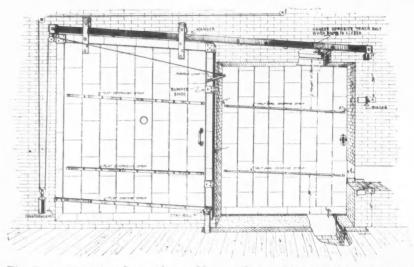
Fire Doors, Dividing Large Areas, Mean a Greatly Reduced Fire Risk and Insurance Premiums. An installation of the sliding type is shown here.
