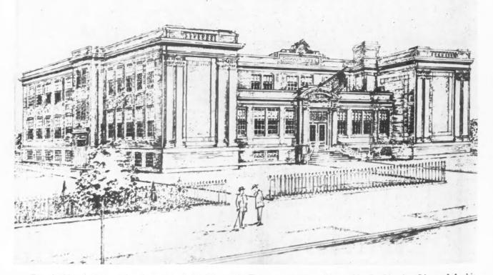
The Architect's Perspective Drawing of the Champlain Elementary School Shows Simple, Pleasing Lines of Architecture and Carefully Studied Orientation Providing a Bright, Cheerful Interior. The light in each class room is arranged to come from one direction only.
