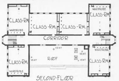
The Second Floor Plan of the Champlain School Shows Six Class Rooms of Uniform Size and a Corridor Which Is Daylighted Throughout Its Length. The inside walls of the front wings are purposely left blank so that the class rooms may receive light from one direction only.
