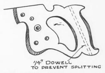
Carpenters Will Be Saved Many a Broken Saw Handle by Inserting a Dowel as Shown Here.
