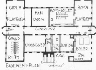
The High Basement of the Champlain School Is Really a Ground Floor and Has Plenty of Light and Ventilation. The floor plan shows two large playrooms and two toilet rooms on this floor as well as boiler and fan room, janitor and electrician's rooms.
