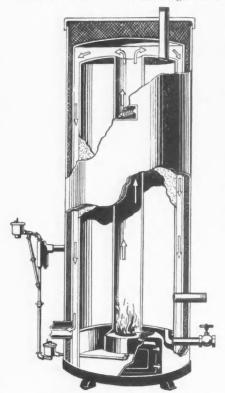
Here Is an Automatic Water Heater Using Oil Fuel Which Can Be Converted Into a Gas Burner Almost Instantly.
