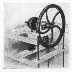
Here Is Shown the Elevating Mechanism of a Dumbwaiter Design for Apartment House Installations and Supplied Complete, Ready for Erection.
