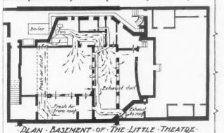
Showing fresh air and exhaust ducts and plenum chamber. Black arrows show fresh air distribution and red arrows show foul air.
