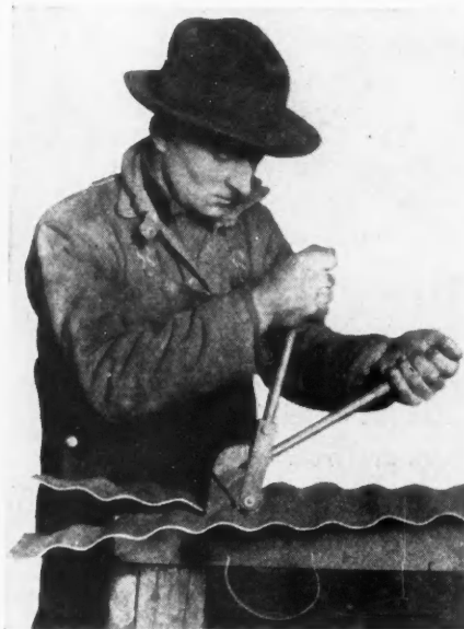
Corrugated Sheet Metal Can Be Cut Right on the Job with This Light, Handy Tool without Distortion.
