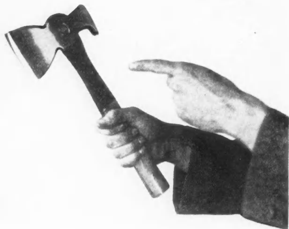
The Head of This Hatchet Can Never Fly Off for It Is Forged, Together with the Handle, in One Piece, Assuring Complete Safety.
