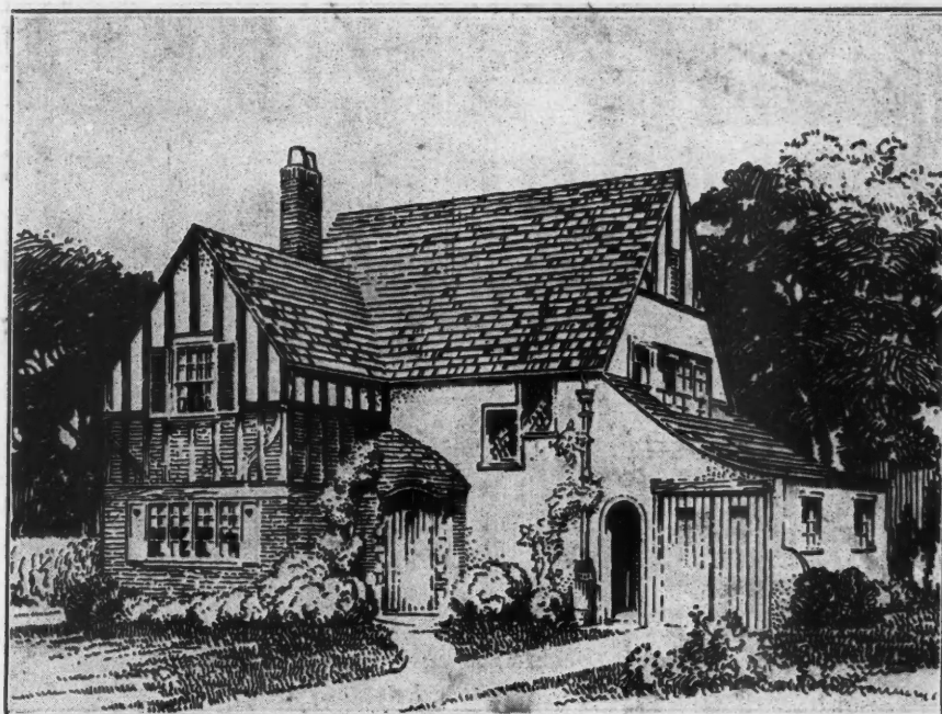
A Six Room, Elizabethan English, Half Timbered, Stucco House of Frame Construction With Common Brick Veneer and Wood Trimmed Exterior from the Plan Shown Below.
