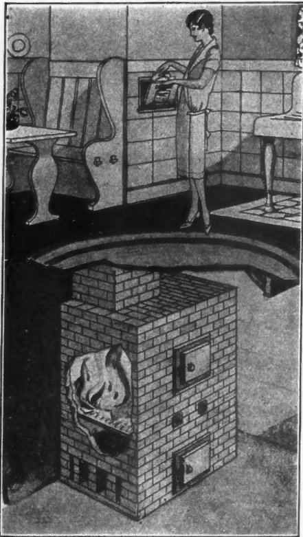
A Built-In, Chute Type of Incinerator Which Can Be Installed Satisfactorily in Buildings of Any Height.
