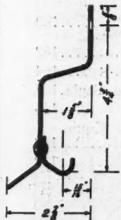
Above is an end view of a piece of "Glide" Track with all dimensions given. Notice the wide running space for the Hangers.
