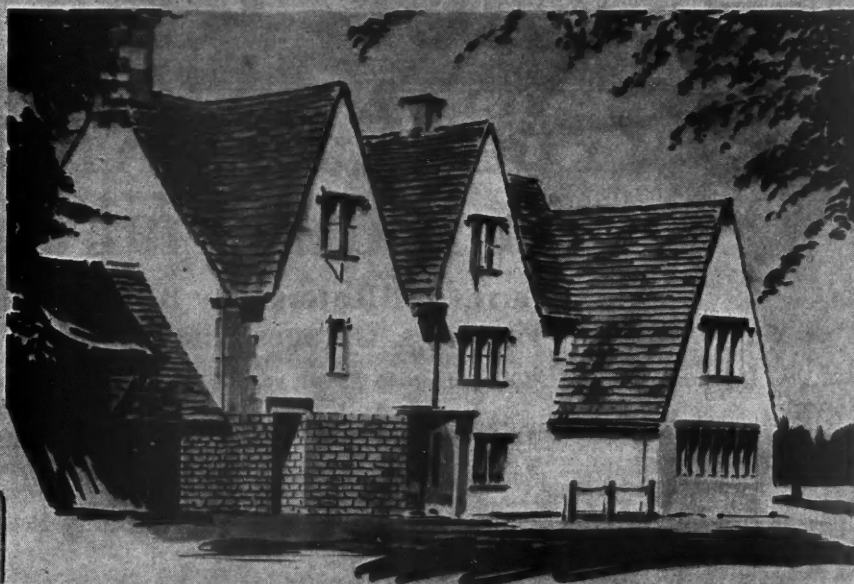
FIG. 1. A SPLIT STONE ROOF OF THE COTSWOLD DISTRICT. A VERY ATTRACTIVE, COLORFUL AND SUBSTANTIAL ONE FOR STEEP PITCHES. SAME EFFECT CAN BE GAINED WITH HEAVY RAG-EDGE FIRE-PROOF SHINGLES LAID TRIPLE AT THE EAVES AND BOUND OVER AT THE GABLE ENDS.
