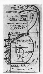
This Sketch Shows the Construction of the Electric Fireplace Heater.
