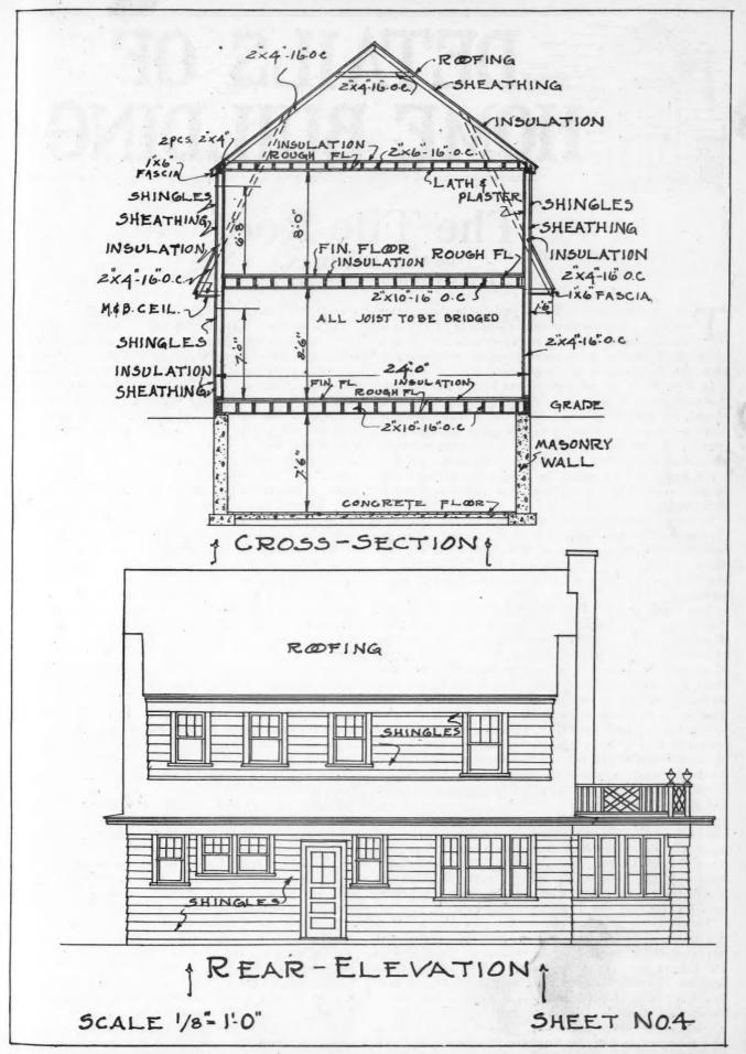
Floor, Roof and Wall Construction, with Thorough Insulation Indicated, Are Seen in the Sectional View While the Rear Elevation Completes the Story of Our Front Cover Home.
