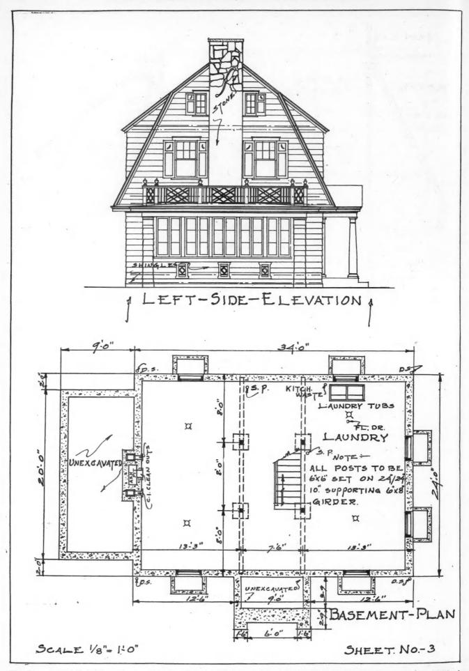
The Basement of Our Front Cover Home Is Completely Excavated and Affords Space Which Can Easily Be Utilized if Extra Rooms Are Desired. The elevation shows the placing of the fireplace chimney.
