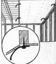
Both Time and Labor Are Saved in the Erection of Wallboard Ceilings by the Use of This Hanging
