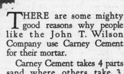
Carney Cement takes 4 parts sand where others take 3. One man can easily furnish mortar to 30 masons, because he is not bothered with soaking and lime is not needed. The extreme plasticity and gradual setting quality of Carney Cement Mortar stops mortar wasting and gives the masons a bigger day -they are not hampered by tamping and tempering on the boards.
