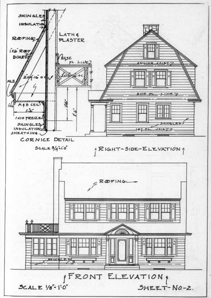
These Elevations Show the Front and Right Side of the House While the Detail Drawing Indicates the Construction of the Cornice. The following pages tell more of the construction story.
