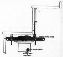
With This Switch Installed You Need Never Worry About Whether You Remembered to Turn Off the Cellar Light.
