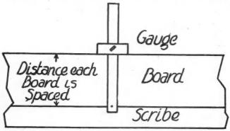
By Means of an Ordinary Wood Gauge, Siding Can Be Marked and Laid True and Straight Quite Rapidly Without Danger of Error.
