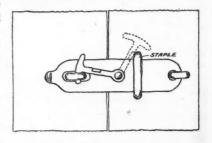
Convenience in Hooking the Hasp, Even When Carrying an Arm Load Is Possible by This Little Device.
