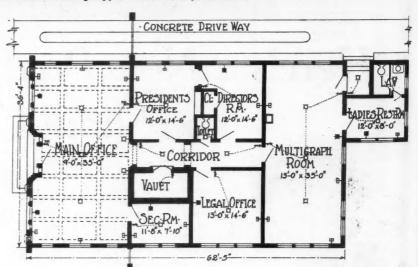
The Office Space Provided Can Be Increased When Required by the Addition of a Second Story, Foundation Construction Having Been Planned with This in Mind.
