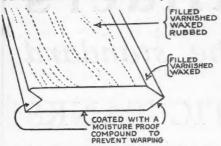
This Sketch Shows How the Ready Finished Flooring Is Treated to Prevent Warping.
