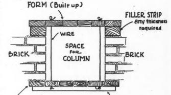
By This Plan the Brick Wall Is Built First and Serves as a Part of the Concrete Column Form.
