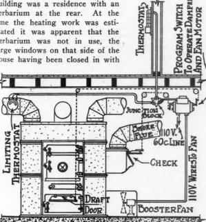
One of Two Accepted Methods of Applying Thermostatic Regulators in Warm-Air Heating Systems, Showing the Dual Control.
