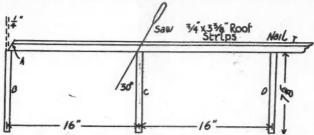
Bridging to Go Between Joists Can Be Cut to Fit Quickly and Accurately by the Method Described and Illustrated Here and a Little Practice Will Increase the Speed of the Work.
