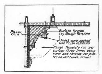
Fig. 2. Diagram Showing the Relation of the Surface Formed by the Rough Template to That Formed by the Finished Template.
