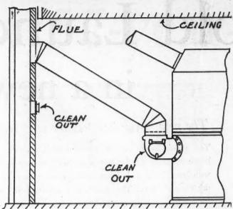
Fig. 3—A Better Method Is a Sloping Smoke Pipe; Better Draft and Freedom From Soot Accumulation Are Thus Provided.
