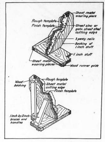
Fig. 4. The Finish Template Cutting Edge Nailed Over the Rough Template Cutting Edge.
