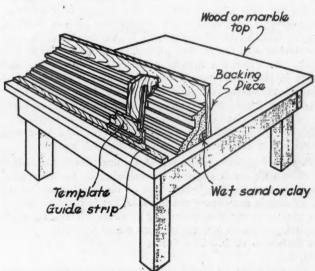
Fig. 7. Table for Running Cornices to Be "Stuck" in Place as in the Corner Shown in Fig. 6.
