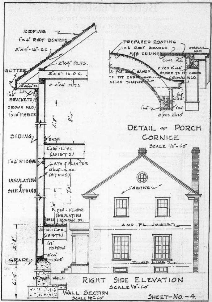
Details of Wall Section and Cornice Show the Elements of Good Construction Found Throughout Our Front Cover Home.
