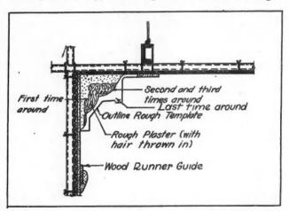
Fig. 1. Diagram Showing the Various Steps in Building Up a Cornice to the Outline of the Rough Template.
