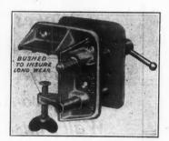
This Woodworkers' Vise, Because of Its Aluminum Construction, Is Extremely Light, Weighing Only 2½ Pounds.
