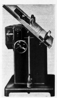
This Motor on Arbor Machine, Operating from the Lighting Circuit, Incorporates Many Improvements.
