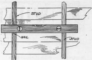
This Method of Testing a Level Is Simple and Exact.
