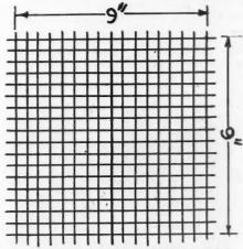
Mesh Wire Piece of 1/2-Inch Cloth Makes an Excellent Scratcher for Stucco.
