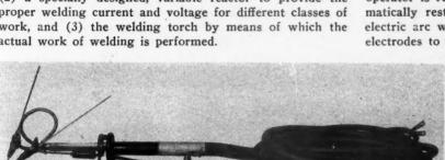
A Close-Up View of the Torch Used in the New Atomic Hydrogen Welding Process.
