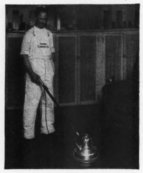
Here Is a Simple Electric Floor Machine That Scrubs, Waxes, Polishes, Buffs or Removes Old Floor Finishes.
