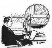
This Ventilator May Be Installed in Any Window and Acts Automatically When the Window Is Opened.
