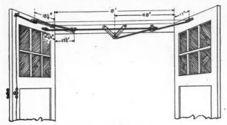
Here Is a Simple and Reliable Piece of Garage Door Equipment Which Makes It Possible to Open Both Doors at Once and Have Them Stay Open.
