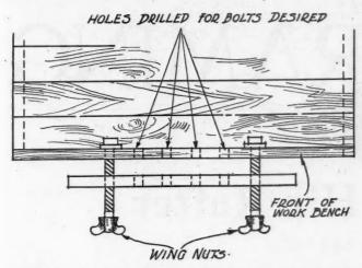
This Special Vise Added to a Work Bench Will Handle, to Best Advantage, Certain Work for Which the Regular Vise Is Not Adapted.
