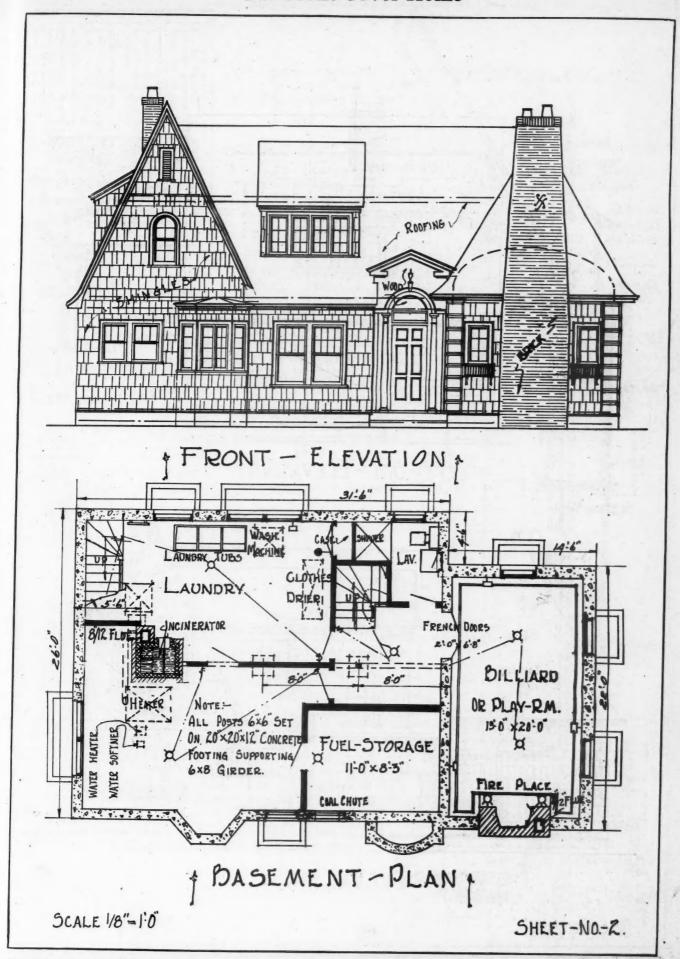
Here We Have the Basement Plan and Front Elevation and Find That Basement Space Has Been Utilized to Provide an Extra Room. Further elevations and details are shown on the following pages.
