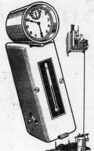
A Simple and Reliable Furnace Control Which Automatically Opens the Drafts in the Morning Without Attention.
