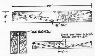
A Steel Rod, Used as Shown Here, Makes a Beam Which Can Be Depended Upon Not to Sag.
