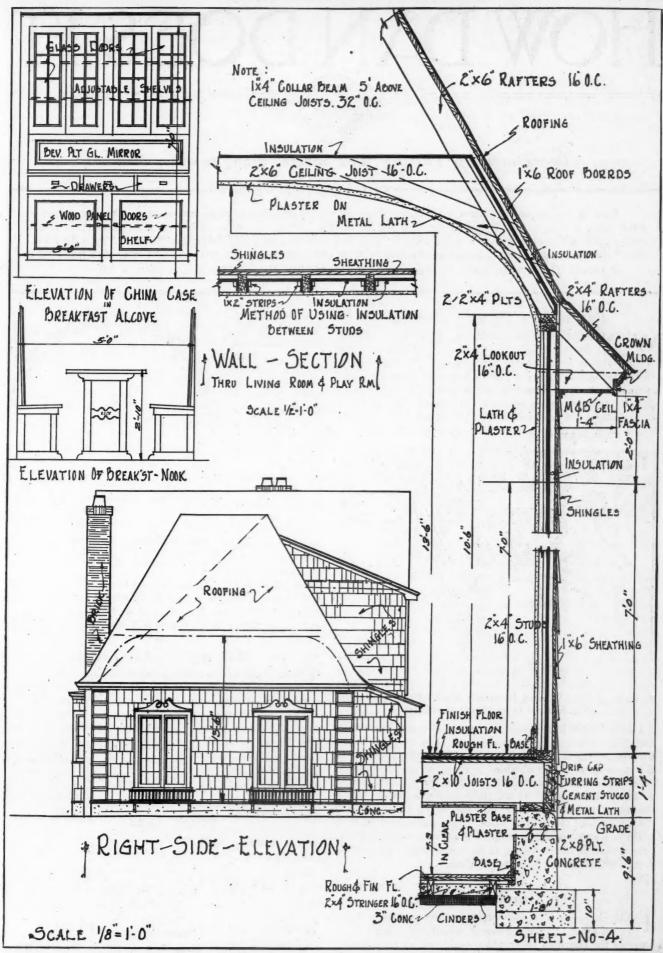
Construction Details of the Arch Ceiled Living Room, a Wall Section and Elevations of the Breakfast Nook and Its Built-in China Case as Well as One More Side Elevation of Our Front Cover Home.
