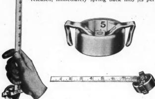
Something Entirely New in the Way of a Rule. It is of steel stiff enough to be extended from one hand as shown, but so flexible under a certain stress that it can be coiled in the small, vest-pocket container shown above.
