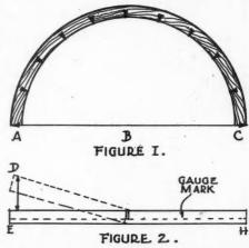
Fig. 1 Shows a Board Kerfed to Fit an Arch. Fig. 2—The Method of Finding the Distance Between Kerfs.
