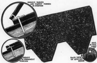
Here Is a Composition Shingle of the Hex Type that Is Designed to Resist the Most Severe Wind Storms.
