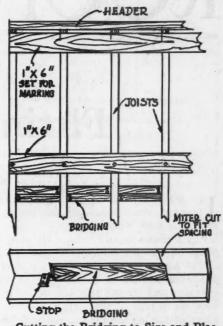
Cutting the Bridging to Size and Placing in This Way Takes the Bows and Twists Out of Joists.
