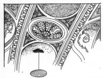
A Piece of Tin, Painted to Match the Ceiling and Drawn Up Against It by Means of a Cord.
