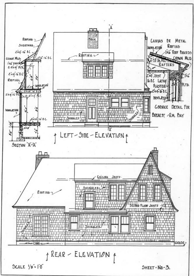
Two More Elevations of Our Front Cover Home and Construction Details of the Outside Walls and the Cornice for the Breakfast Room Bay Are Shown Here.
