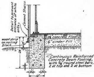
A Continuous, Reinforced Concrete Beam Footing Suitable for Houses and Other Small Buildings Without Basements.
