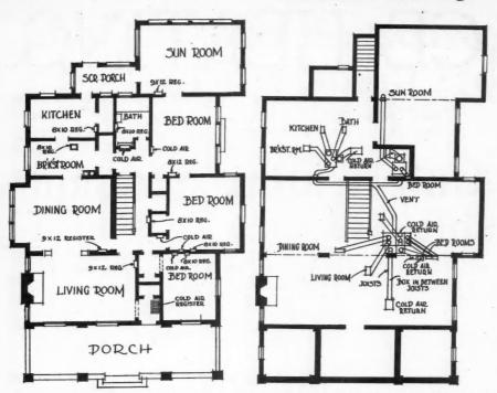
Fig. 2—Floor and Basement Plan Illustrating the Proper Method of Grouping Gas-Fueled Heating Units of the Type Discussed in This Article.
