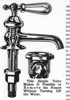
The illustration shows this device and how it is installed in the faucet. It can be used with any type of faucet and conforms to the most modern plumbing practice. The device consists of three parts. There is a brass housing threaded to screw into the faucet, forming the seat. This housing contains a non-corrosive steel ball. which is forced up by the pressure of water against an air tight seat (in the brass housing) and automatically
