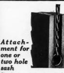
Simply drop chain through the bore, slip coil spring into end link, give the coil a turn and insert in sash with thumb. For two hole sash, insert coil in upper hole
