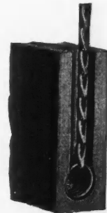
For one-hole sash, a coil spring provides a strong grip that cannot tear loose. Simply slip coil into end link, give it a turn and insert in sash with thumb.
