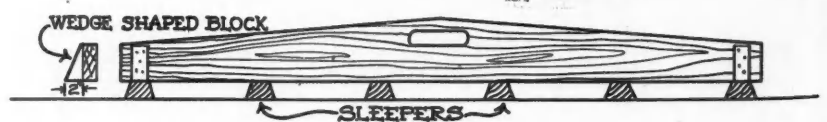
Wedge-Shaped Blocks Nailed to the Long Straight Edge Used in Laying Sleepers Will Keep Them from Being Blown Over on a Windy Day.
