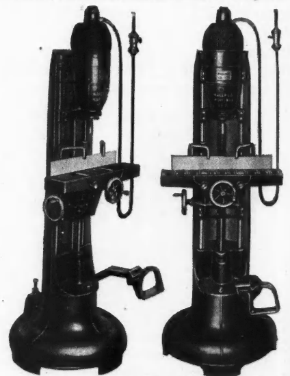
This New, Portable, Hollow Chisel Mortiser Can Be Used for Square Holes Up to \frac{1}{2} Inch.
