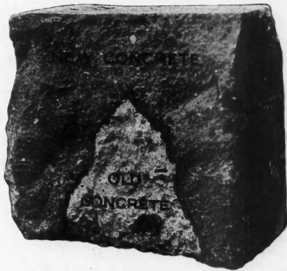
New Concrete Bonded to Old Concrete with This Compound Makes a Joint as Strong as the Original Cast.
