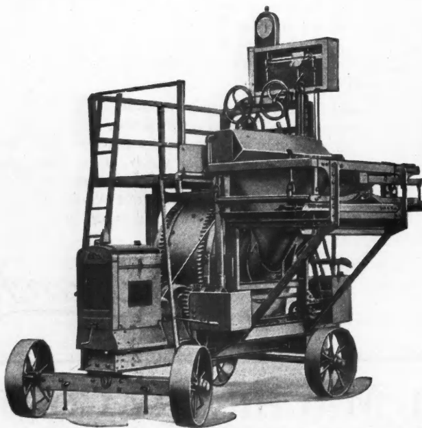
This Mixer, Equipped with a Weighing Batch Hopper and Water Tank, Makes Possible Accurate Proportioning of Materials.
