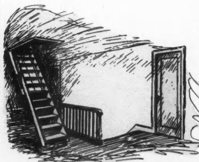
The disappearing stair to the attic is a modern improvement, useful in most homes.
