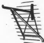
Trouble Saver Nail Attached Brackets support a ton. Held by four nails.
