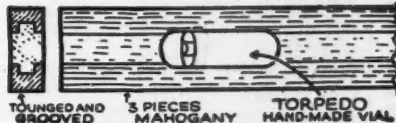
Above: The Torpedo Shaped Vial Used in the New Level Construction of Which Is Shown Below.
