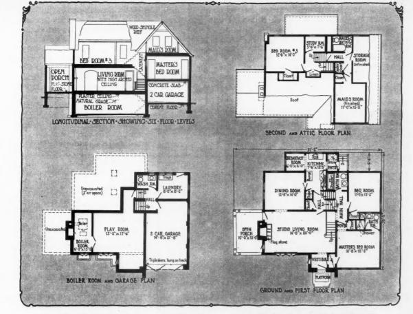
A Most Unique Arrangement for a Home to Be Built on a Sloping Site Is Presented. The Rear or Garage Section Is a Half-Story Above the Main Wing on Every Floor, Making Six Levels, Each Reached by a Half-Flight Stair
