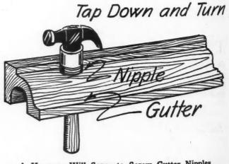
A Hammer Will Serve to Screw Gutter Nipples Into Wooden Eave Trough.
