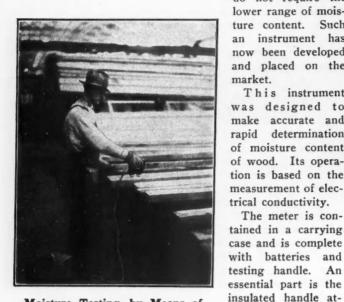
Moisture Testing, by Means of a Meter. A workman is applying the testing handle to lumber.
