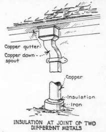
to the track was subject to corrosion. The grounded current "strayed" away from rails, which were not then well bonded, and to some extent passed through the piping. The action is possible in building where galvanic action is set up between two metals by the aid of moisture. Copper and steel for instance. Copper gutters and down-spouts should not be joined to steel or iron piping without thorough installation.
