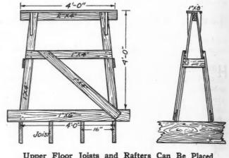
Upper Floor Joists and Rafters Can Be Placed with the Aid of This Trestle.
