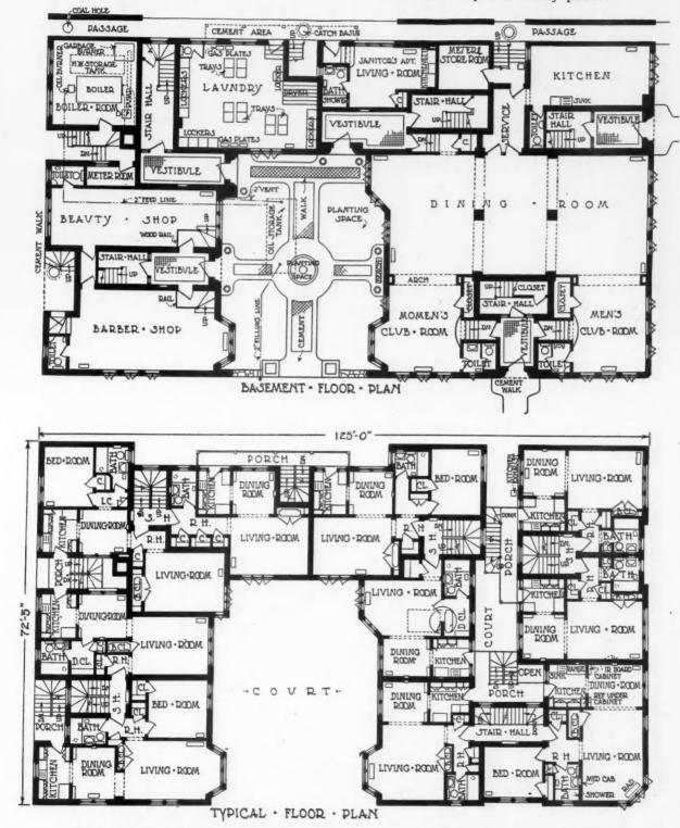
The Plans of This Apartment at Harvey, Ill., Designed by John T. and Murray D. Heatherington, Architects, Show an Effective Use of Space-Saving Equipment, and an Interesting Utilization of Basement Space.
