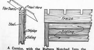
Cornice, with the Rafters Notched Into the Frieze Board, Makes a Weather-tight Job. and cut notches carefully so that the rafters will fit into them snugly. Put the rafters down deep enough into the . notches, so that you can dress off, with a plane, the upper edge of the frieze board.
