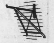
Trouble Saver Nail Attached Brackets support a ton. Held by four nails.
