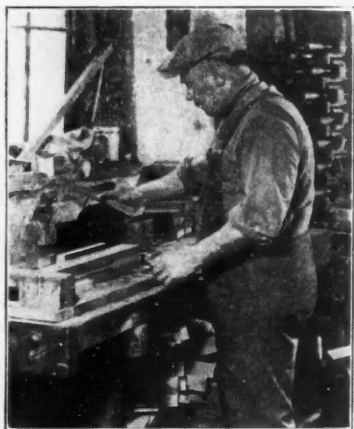
Mixed with Cold Water and Used Cold This Glue Is Not Affected by High Moisture Content in Wood.
