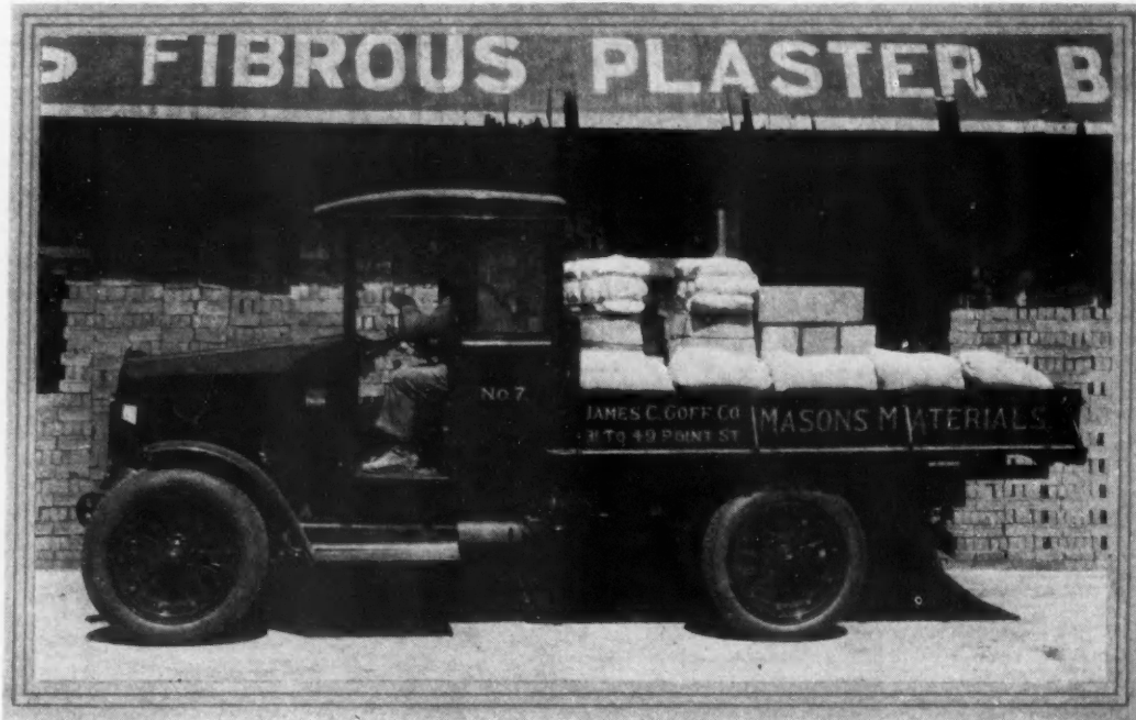
Place the Greatest Part of the Load Toward the Front of the Truck Body
