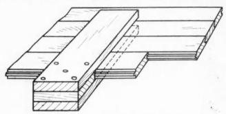
A Simple Means of Holding the End of Ceiling, While Nailing, Which Makes a Helper Unnecessary.
