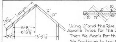
Wing 12" and the Rive Per Foot Run On the Javare we Apply the Javare Twice For the 2 Feet Run Of Tail.
