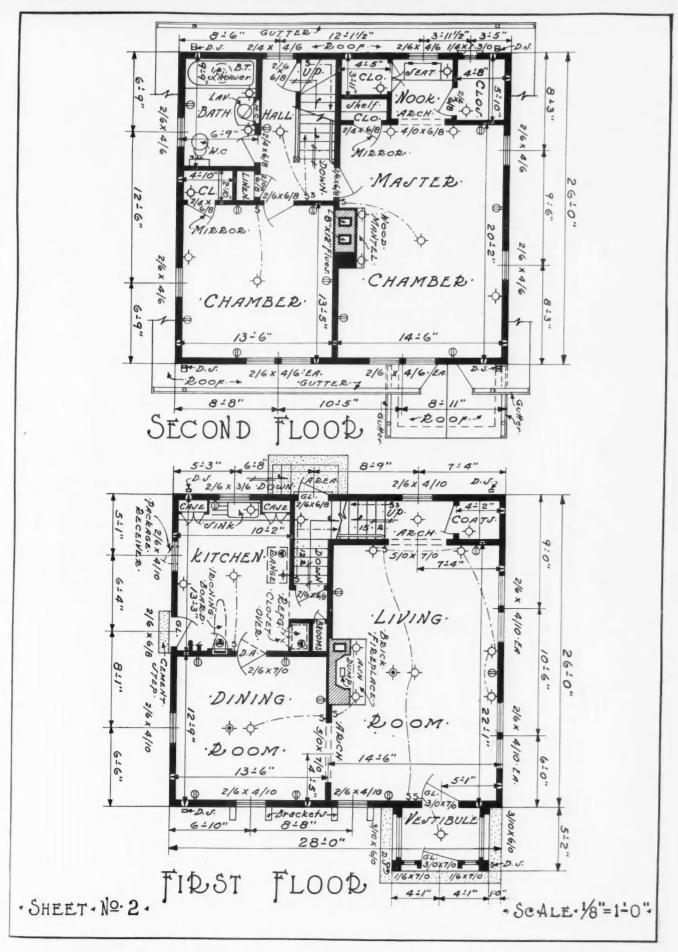
Notice How Every Bit of Space Is Utilized in This Plan; a Raised Blanket Closet Is Worked in Above the Main Stair Without Sacrificing Head Room. Elevations follow.
