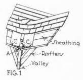
Construction for Filled Valleys with Composition Shingles.
