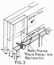
Construction of a Batten Door for the Living Room to Outside.
