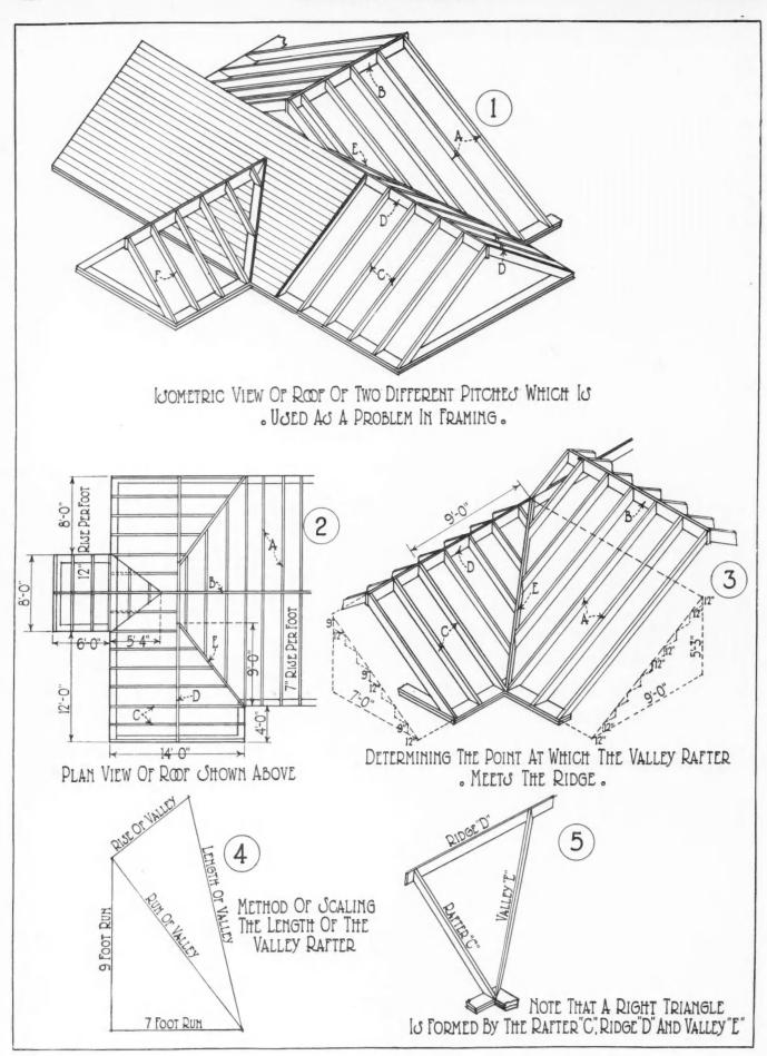
Diagrams Showing How to Handle a Roof of Two Different Pitches.
