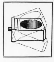
**THIS is the exclusive NORWALK Self**. Adjustable Strike that engages bolt from any angle, locks the door regardless of shrinkage, warp or sag.
