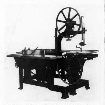
A Universal Woodworking Machine Which Eliminates the Use of Clutches for Starting and Stopping.
