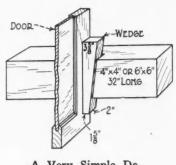
A Very Simple Device for Holding a Door While Working on It.
