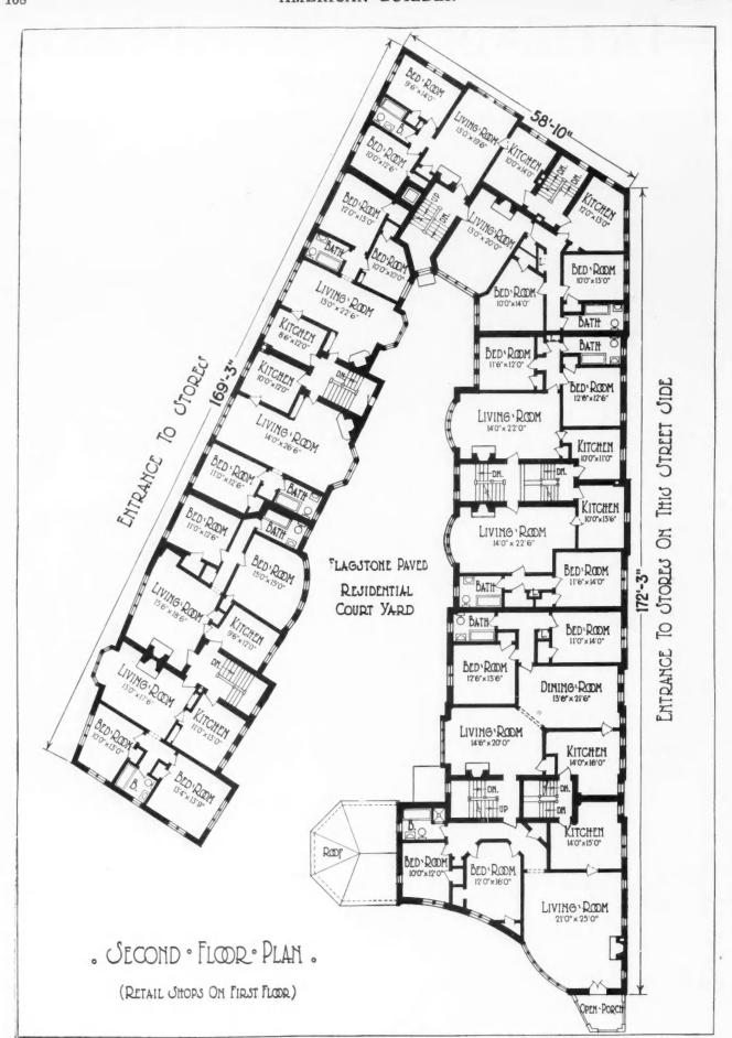
"THE CHIMNEYS," Winnetka, Illinois. Second floor plan of this distinctive apartment building, built in Tudor architecture around a triangular shaped court.
