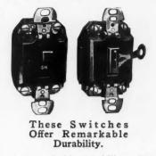
these switches to be of uniformly remarkable durability. The cups being especially shallow, 1 15/16 inches, ample wiring space is provided, and, due to construction and special bakelite stops, these switches are unusually quiet in operation. All switches of this series can be supplied with a luminous insert or lock type handles.
