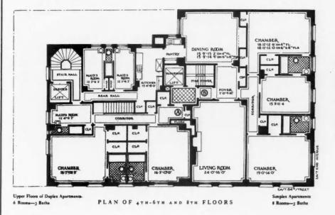
An Unusual Feature of This Building Is the Combination of Entire Floor Apartments, as on the 9th and 10th Floor Plan Above, and Duplex and Simplex Apartments, as on the 4th, 5th, 6th and 7th Floor Plans, Below and at the Left.
