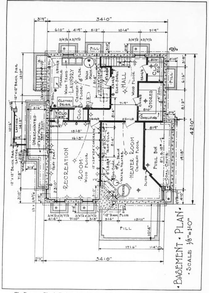
The Basement Plan is Typical of the Modern Trend of House Design, with Every Inch of Space Utilized and Every Room Fully Equipped.
