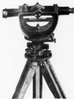
A Transit - Level with Special Features Appealing to the Builder.
