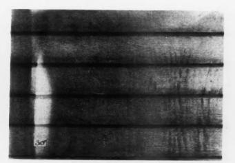
One Coat of Aluminum Paint After 3½ Years on Rough Lumber. Excellent condition; with no visible failure over knots.
