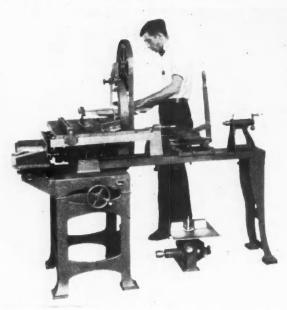
Eight Woodworking Machines in One, the Units of Which Can Be Purchased Separately and Added as Needed.
