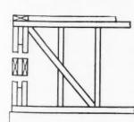
Cutting the brace at a little less than a 45 degree angle adds to the efficiency of the brace; for a brace cut at too flat an angle has a tendency to kick out at the bottom whereas the one at a 45 degree angle must necessarily lift its own weight before the corner will give. Fit the brace to a position against the stud as shown; the upper end
