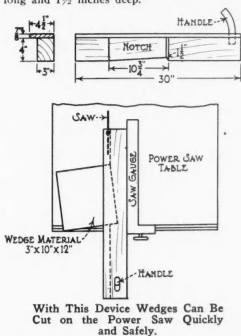
On top of this piece I nail a 7/8 by 41/4 by 30-inch piece. This projects 11/2 inches over the notch and forms a guard. I then make a mortise, for a handle, in the end farthest from the notch. I make the handle with a little curve forward to fit the hand.
